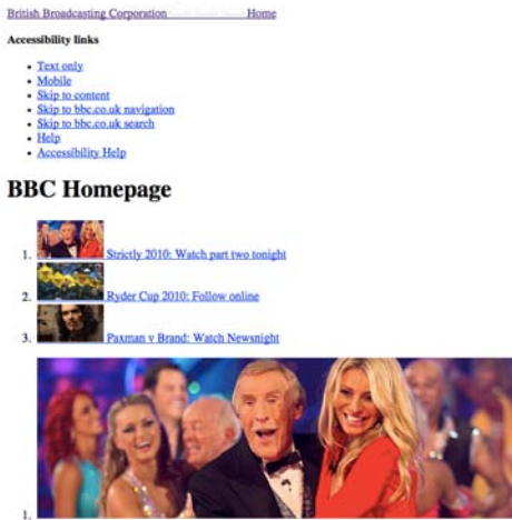
Figure 3-1. The homepage of bbc.co.uk with only the user agent style sheet applied (that of Firefox, in this instance).
