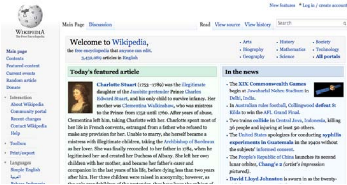
Figure 3-2. The front page of Wikipedia with a user style sheet applied: in this case, the user style sheet ensures that the text on any website is never smaller than 18px.
