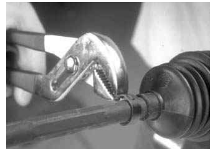
P12-3 Remove the inner and outer boot clamps.
