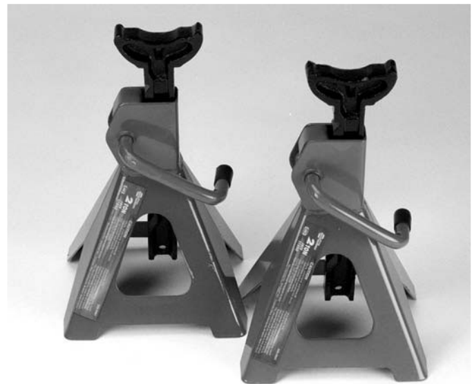
Figure 2-38 Typical safety stands.
