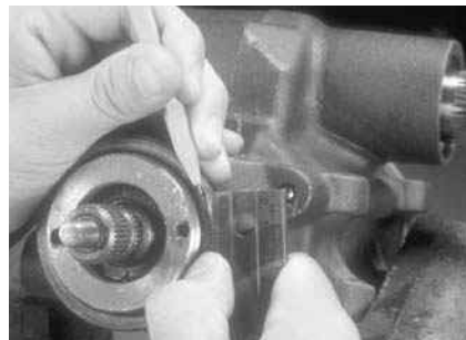
P11-5 Measure 0.50 in. (13 mm) counterclockwise from the mark placed on the housing in step P11-4, and place a second mark on the housing.
