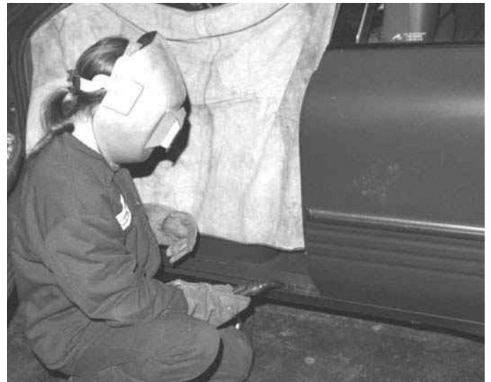
Figure 14-4 Protect the interior and exterior of the vehicle while arc welding.
