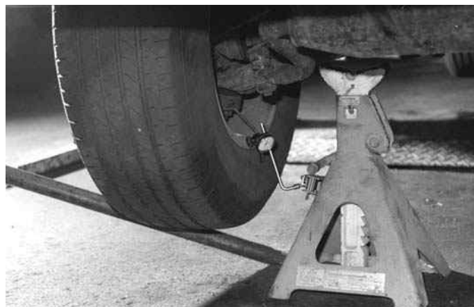
Figure 6-10 Dial indicator installed to measure vertical ball joint movement on a compression-loaded ball joint.
