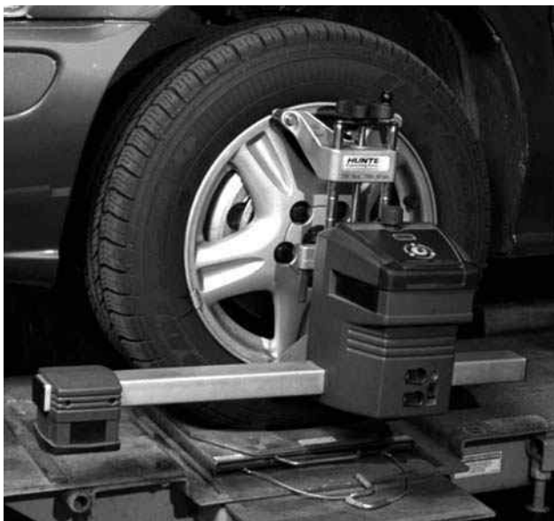
Figure 15-14 Cordless wheel sensor containing a high-frequency transmitter.
