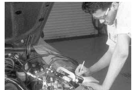
P10-9 Check and record the power steering pump pressure at 3,000 rpm.
