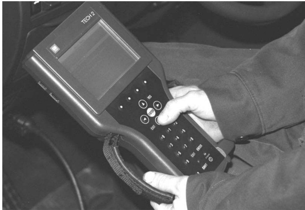
Figure 2-32 Scan tool for diagnosing computer-controlled suspension systems.
