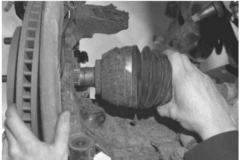
Figure 6-33 Removing the drive axle from the axle hub.
