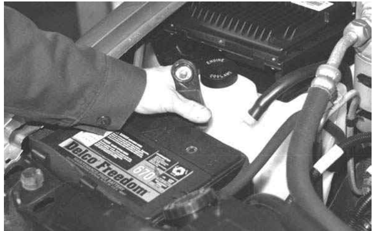
Figure 14-2 Remove the negative battery cable before arc welding on a vehicle.
