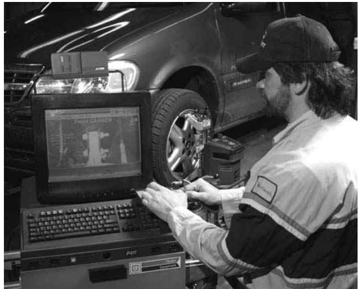
Figure 15-15 Computer wheel aligner with data receiver on top of the monitor.
