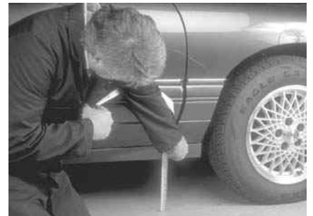
P7-6 Measure and record the left front curb riding height.
