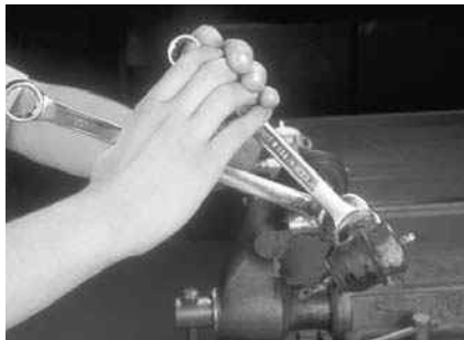
P12-2 Loosen the jam nut and remove the outer tie-rod end and jam nut.
