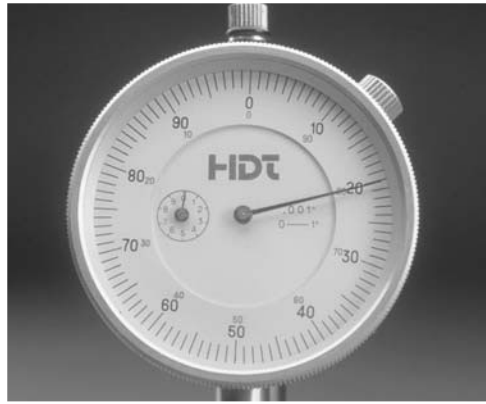
Figure 2-41 The dial indicator pointer rotation indicates the amount of plunger movement.
