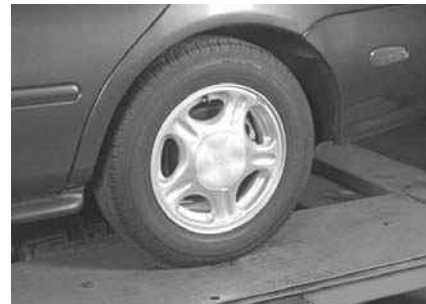
P15-3 Position the rear wheels on slip plates.
