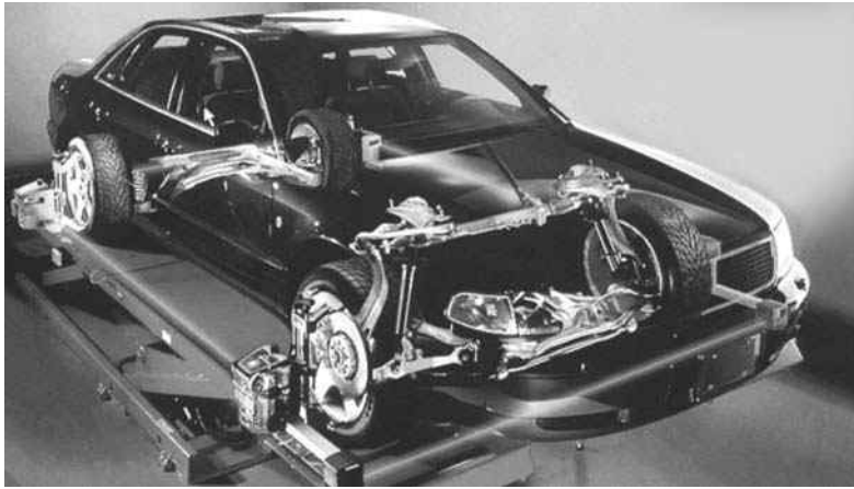
Figure 15-16 Front and rear wheel sensors with optical arms.
