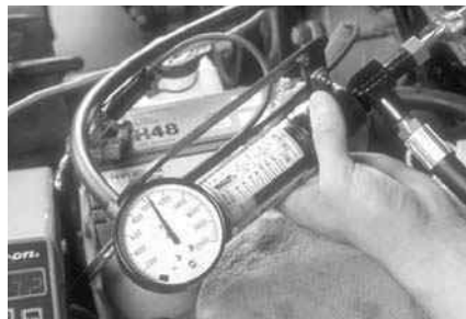
P10-10 Check and record the power steering pump pressure with the steering wheel turned fully in one direction and the engine idling.
