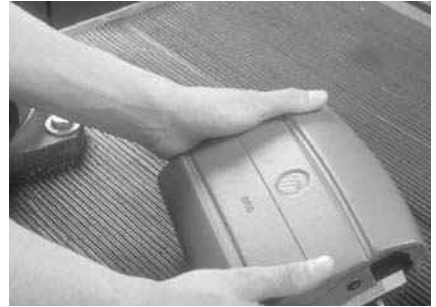
P9-6 Set the air bag deployment module face upward on the workbench.
