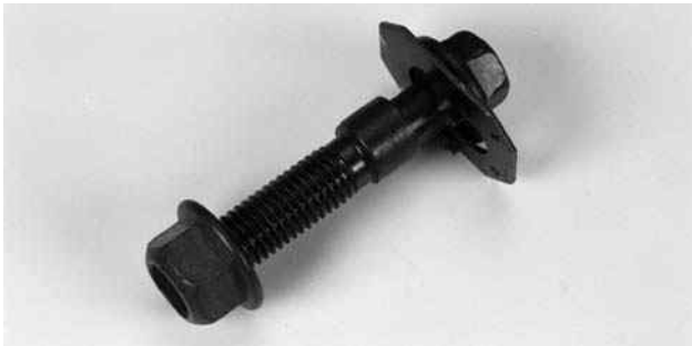
Figure 16-9 Camber adjustment kits provide 2\frac{1}{2}^\circ camber adjustment on some General Motors cars.
