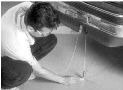
P14-4 Suspend a plumb bob at the manufacturer's recommended frame measurement locations and place a chalk mark on the floor directly under the plumb bob.
