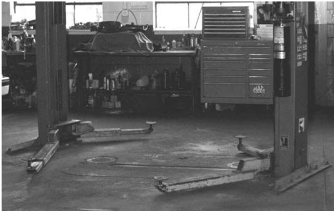
Figure 2-37 Vehicle lifts are used to raise a vehicle.
