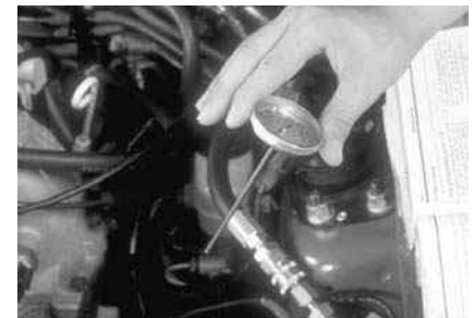
P10-6 Place a thermometer in the power steering fluid reservoir. Be sure the fluid temperature is at least 176°F (80°C).
