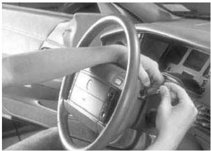
P9-4 Remove the air bag deployment module retaining screws under the steering wheel.
