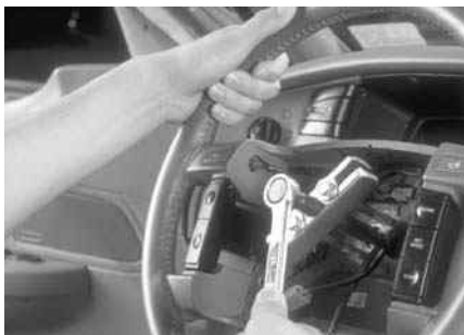
P9-10 Turn the puller screw to loosen the steering wheel on the shaft.
