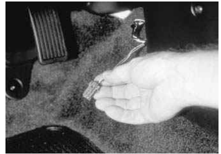
P14-3 Lower the vehicle and locate the service check connector behind the center console.
