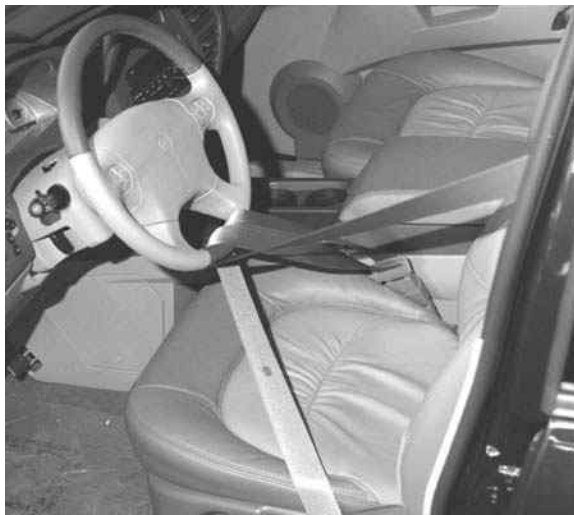
Figure 12-3 Driver's seat belt wrapped around the steering wheel to prevent wheel rotation.
