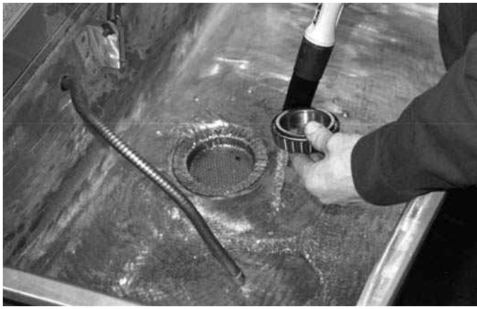
Figure 3-3 Cleaning a bearing with solvent.
