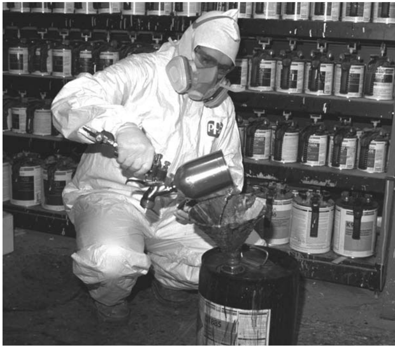
Figure 1-1 Always wear recommended safety clothing and equipment when handling hazardous materials.
