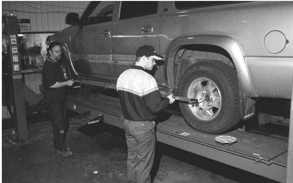
Figure 16-64 Track bar positioned to measure rear wheel tracking.
