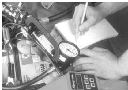
P10-8 Check and record the power steering pump pressure at 1,000 rpm.
