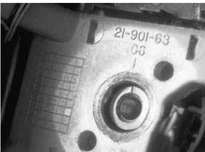
P9-8 Observe the alignment marks on the steering wheel and shaft.
