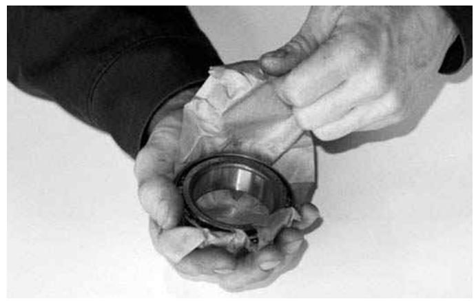
Figure 3-4 Wrapping a bearing in waterproof paper.
