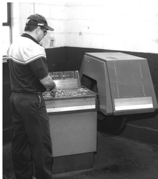
Figure 2-10 Typical electronic wheel balancer.
