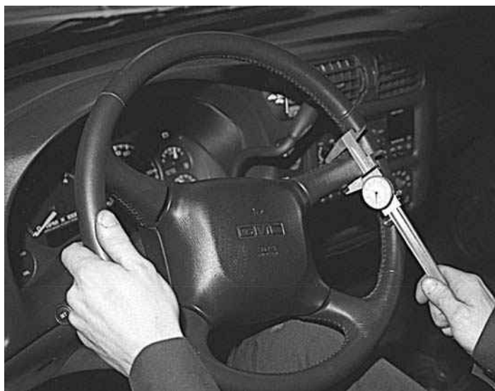
Figure 12-2 Checking steering wheel free play.
