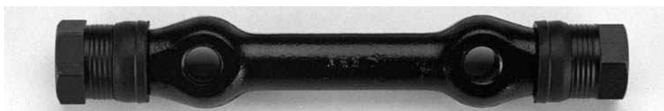
Figure 16-7 Upper control arm shaft kit provides an extra 1 1/2° camber adjustment.
