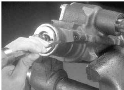
P11-4 Place an index mark on the steering gear housing next to one of the adjuster plug holes.
