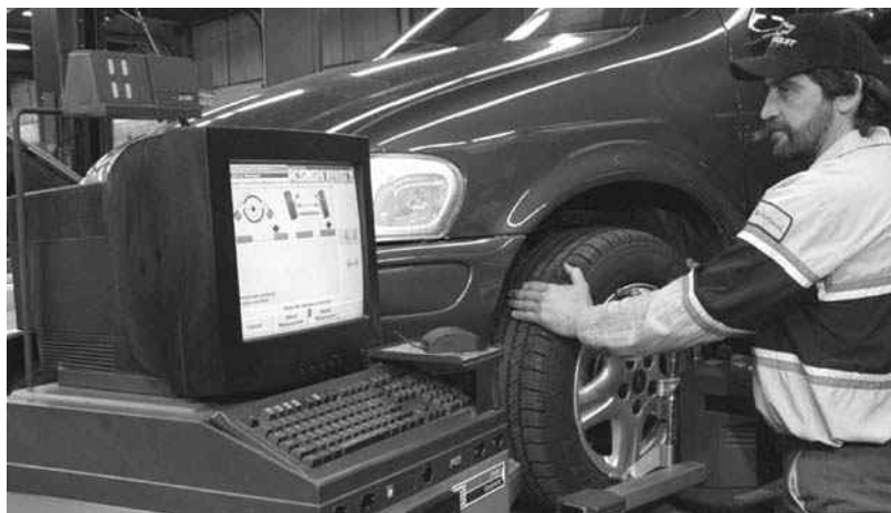
Figure 15-21 Wheel swing procedure illustrated on the screen.
