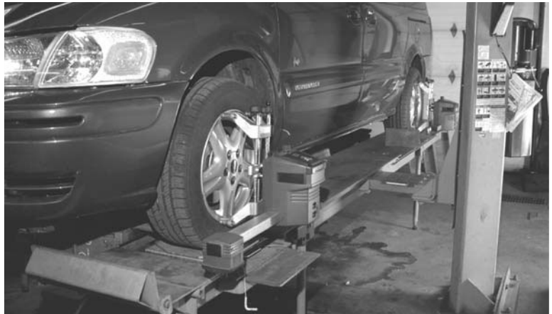
Figure 2-30 Fiber optic track and toe gauge.
