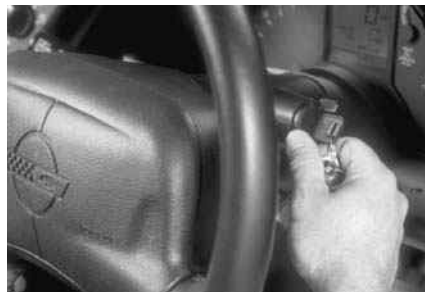
P10-4 Start the engine, and turn the steering wheel from lock to lock three times to bleed air from the system and heat the power steering fluid.
