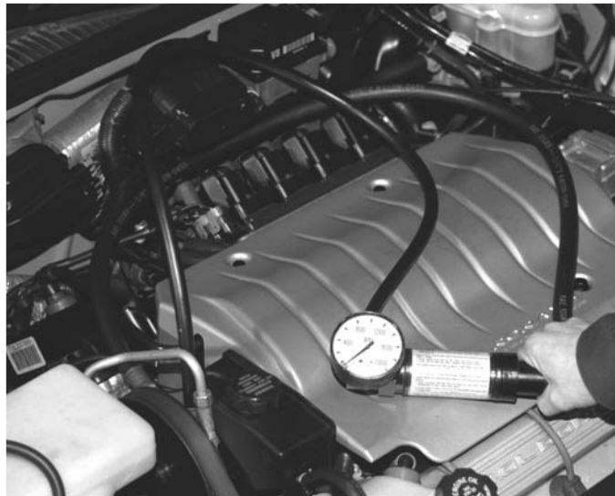
Figure 2-40 Pressure gauge connections to power steering.
