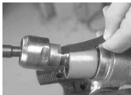
P12-10 Use a feeler gauge to measure the clearance between the rack and the inner tie-rod joint housing stake.
