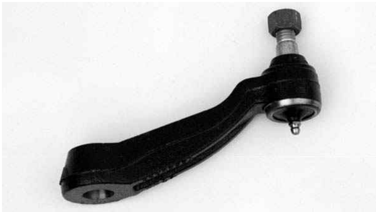
Figure 9-22 Pitman arm design.
