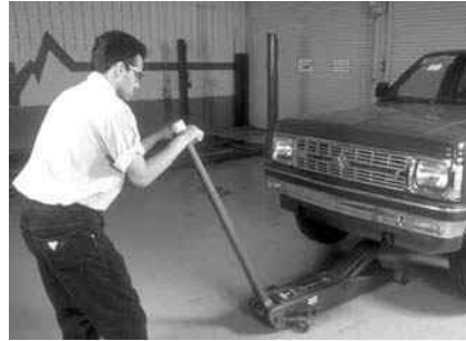
P14-2 Raise the front suspension with a floor jack and lower the chassis onto safety stands positioned at the manufacturer's recommended lifting points.
