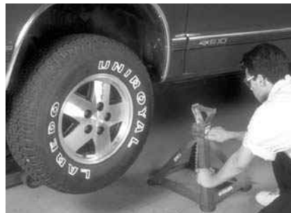
P14-5 Use a floor jack to lift the vehicle, remove the safety stands, and lower the vehicle.
