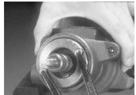
P11-6 Rotate the worm shaft adjuster plug counterclockwise until the adjuster plug hole is aligned with the second mark placed on the housing.
