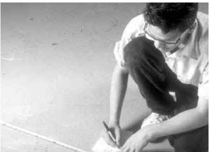
P14-7 Use a tape measure to measure the vehicle's frame measurements between the chalk marks on the floor.
