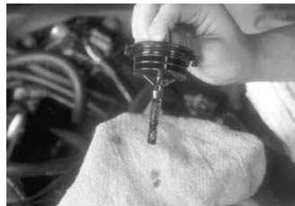
P10-5 Check the power steering fluid level, and add fluid as required.
