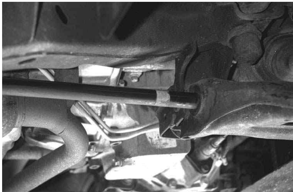
Figure 6-4 Longitudinal torsion bar.
