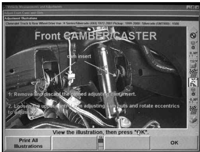
Figure 15-20 Point and click suspension inspection screen.
