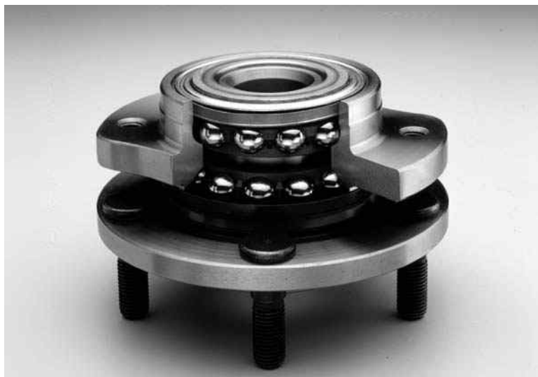
Figure 3-15 Double-row, sealed wheel bearing hub unit.
