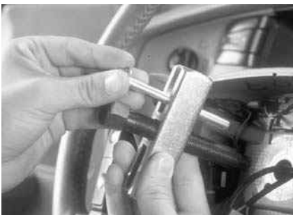
P9-11 Remove the puller from the steering wheel.
