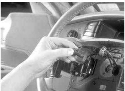
P9-7 Loosen and remove the steering wheel retaining nut.
