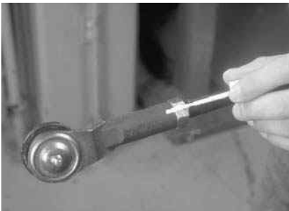
P12-1 Place an index mark on the outer tie-rod end, jam nut, and tie-rod.
