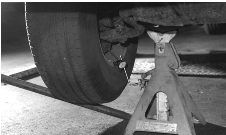
Figure 2-42 Dial indicator installed to measure vertical ball joint movement.
