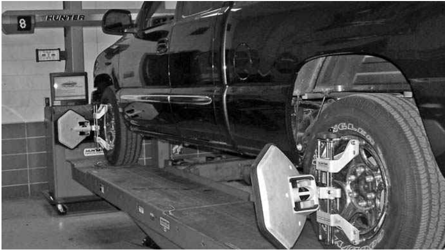
Figure 15-10 Computer wheel aligner with digital cameras and wheel targets.
