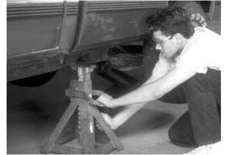
P14-3 Raise the rear suspension with a floor jack and lower the chassis onto safety stands positioned at the manufacturer's recommended lifting points.
