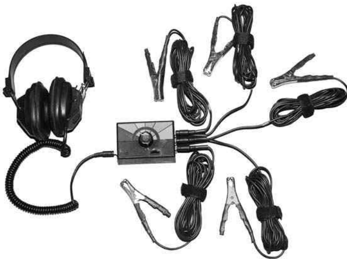
Figure 7-5 ChassisEar tool for locating noise sources.
