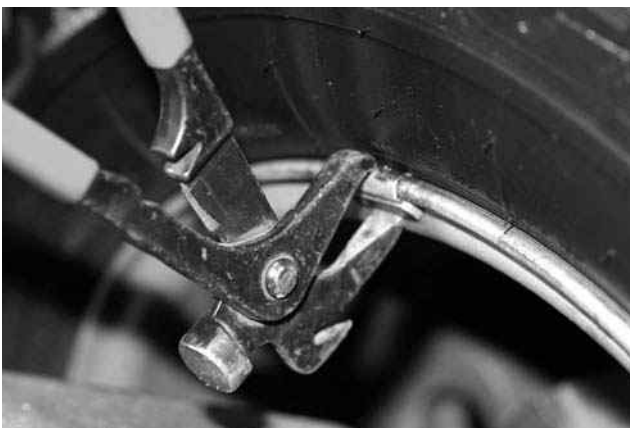
Figure 4-25 Wheel weights are removed and installed with special wheel weight pliers.
