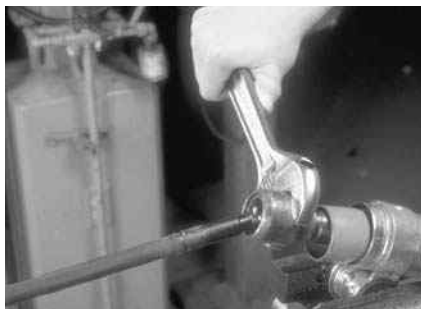
P12-5 Hold the rack with the proper size wrench and loosen the inner tie-rod end with the proper wrench.
