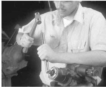
P11-2 Remove the worm shaft bearing locknut with a hammer and brass punch.
