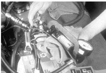
P10-7 With the engine idling, close the pressure gauge valve for no more than 10 seconds. Observe and record the pressure gauge reading.
