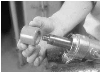
P12-7 Be sure the shock damper ring is in place on the rack.
