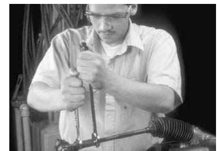
P12-12 Install the jam nut and outer tie-rod end with the index marks aligned.
