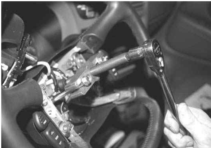
Figure 9-5 Removing steering wheel with the proper steering wheel puller.
