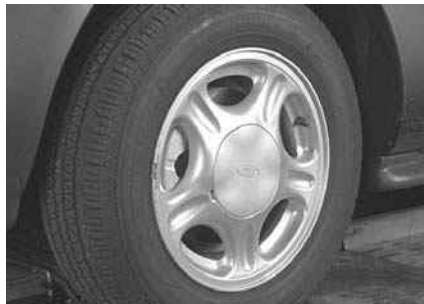
P15-2 Be sure the front tires are positioned properly on the turntables.
