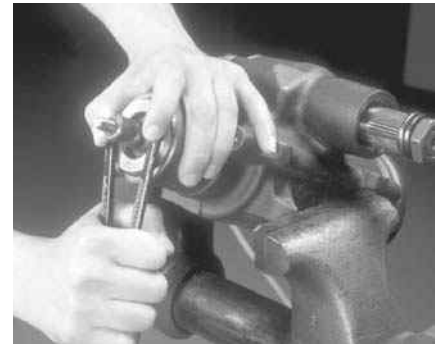
P11-3 Use the proper tool to turn the worm shaft adjuster plug clockwise until it bottoms, and tighten this plug to 20 ft.-lb. (27 Nm).
