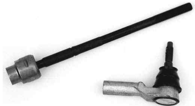
Figure 9-28 Inner tie-rod and outer tie-rod end, rack and pinion steering.
