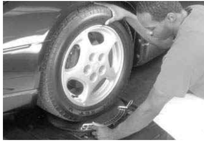
P2-2 Make sure the front tires are positioned properly on the turntables.
