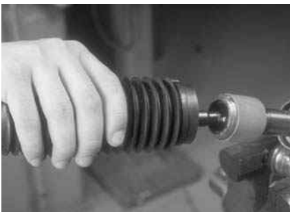
P12-4 Remove the bellows boot from the tie-rod.
