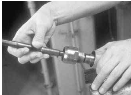
P12-8 Install the inner tie-rod on the rack, and tighten the tie-rod to the specified torque while holding the rack with the proper size wrench.
