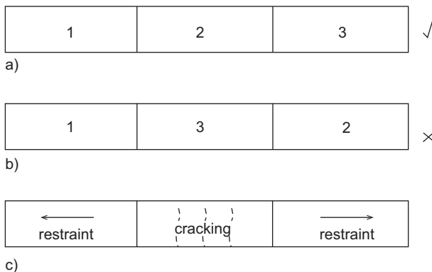
Figure 2.7 Construction sequence (a) Preferred sequence (b) Not recommended (c) Effect of method (b) on third slab panel (cracks shown are illustrative only).
