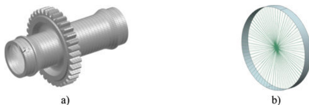
Fig. 2 a FE model of a toothed wheel of an aircraft gear, b the model of support
