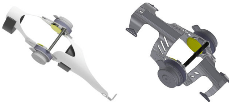
Fig. 4 Robotic orthosis composite and metallic variant
