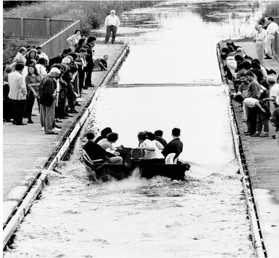
The shallow water soliton on the Scott Russell Aqueduct on the Union Canal near Heriot-Watt University, Scotland, July 12th, 1995.
