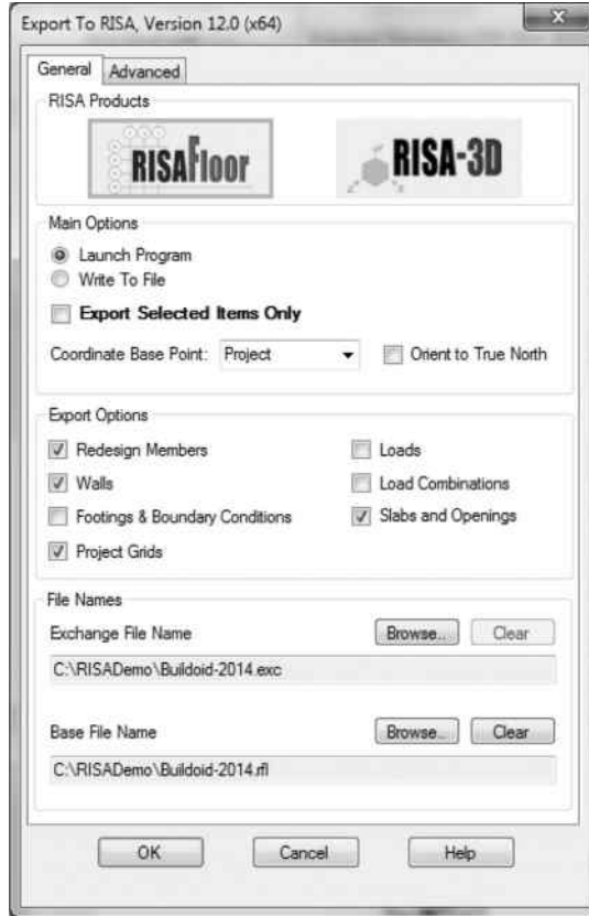
FIGURE 6.39 Direct link to export Revit models to RISA.
