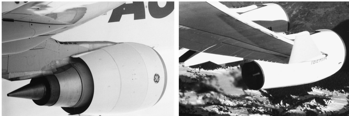
Figure 19.1. An unmixed engine on the Airbus 330 and a mixed engine on the Airbus 340-300
