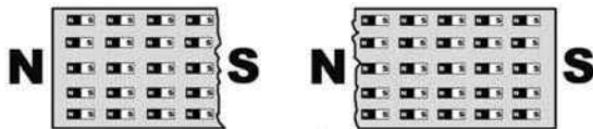
Figure 16.28 broken magnets result in two new magnets, each with its own north and south poles
