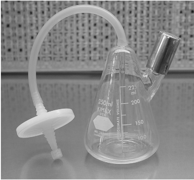
Fig. 1. A modified Erlenmeyer flask used to culture Synechocystis PCC 6803 cells based on an original design described by Williams (4). The 0.2 \mu\text{m} Millipore filter is connected to a glass capillary tube with an outer diameter of 6.0 mm and an inner diameter of 1.7 mm that extends 30 mm above the closed end of the flask and stops 10 mm from the bottom of the flask. The connection is made with Cole Palmer Masterflex tubing. The sidearm is made with glass tubing that has a 20 mm outer diameter and it is covered with a stainless steel culture-tube cap. This whole unit is autoclaved before use.
