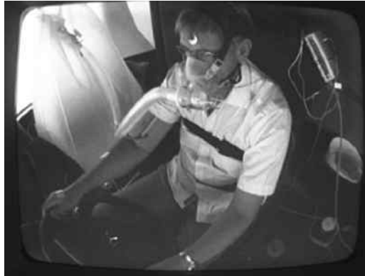
FIGURE 9.12 Experimental analysis of truck driver effort and stress at TRL.
