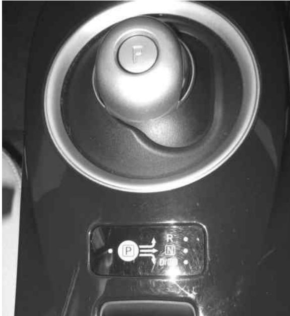
FIGURE 10.8 The drive-mode selector in a modern EV.
