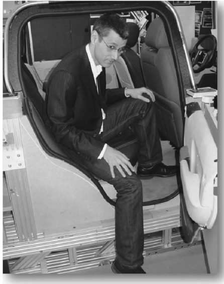
FIGURE 3.15 Taller passenger in a simple buck designed to assess entry to and exit from the rear of a Range Rover.
