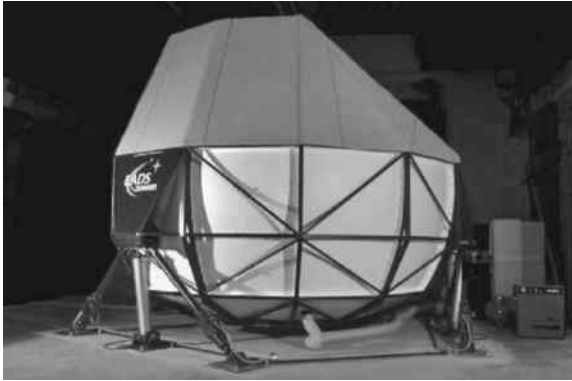
FIGURE 9.8 Full mission truck simulator with advanced motion system.
