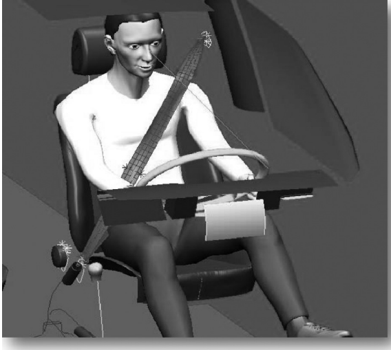
FIGURE 3.12 A male RAMSIS manikin in a representative driving position.
