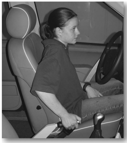
FIGURE 3.16 A shorter female driver assessing the driving position and control placement in a static buck in laboratory conditions.
