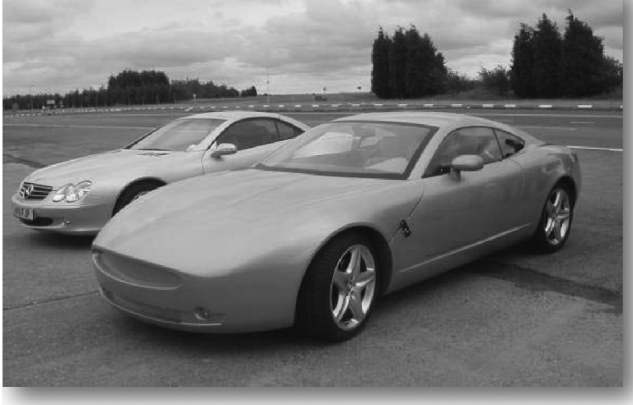
FIGURE 3.17 A dynamic buck with a competitor production vehicle for comparison purposes on the JLR Gaydon test track facility.
