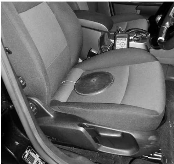
FIGURE 6.4 Flexible disc containing accelerometers mounted on an automobile seat.
