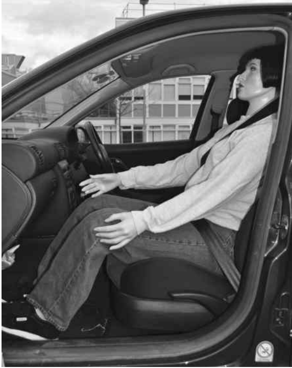
FIGURE 7.3 Thermal manikin ‘Victoria’ in a car.
