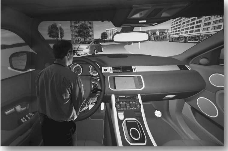
FIGURE 3.14 Range Rover Evoque development in the JLR cave at Gaydon's R and D facility: exterior vision optimised.
