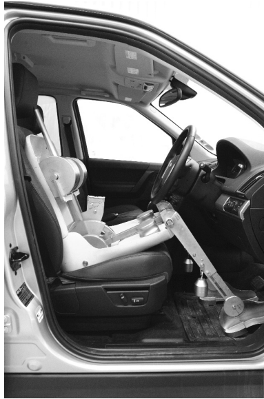
FIGURE 3.8 SAE H-point machine.
