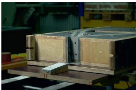
Figure 3.3 Demolding the diamond-shaped element made of textile-reinforced concrete.
