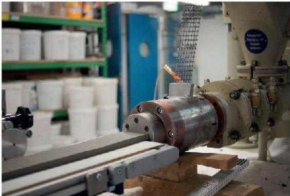
Figure 3.15 Extrusion with feeding device for textiles.
