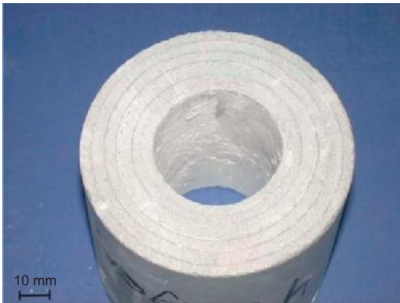
Figure 3.12 Spun tube with four layers of textile reinforcement.
