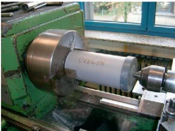
Figure 3.11 Clamped tube during the spinning process.
