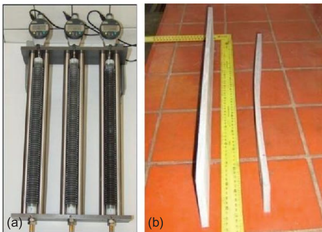
Figure 2.4 (a) Setup for testing autogenous shrinkage; (b) effect of shrinkage on TRC specimen cast with both surfaces facing the formwork (left specimen) and just one surface facing the formwork (right specimen).
