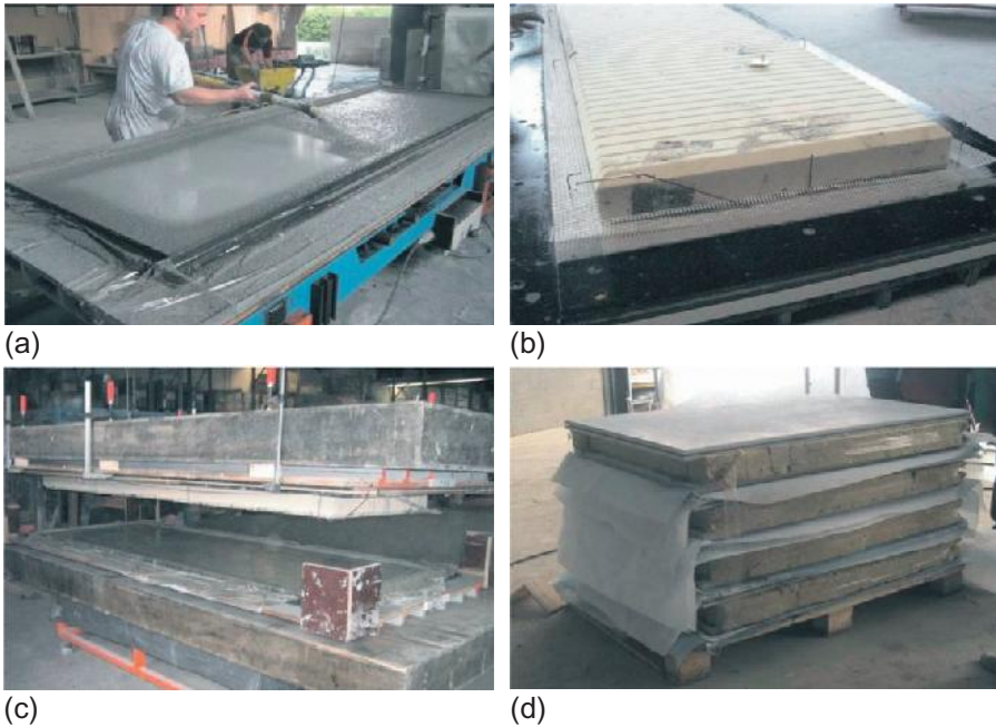
Figure 3.9 Manufacturing a sandwich element: (a) spraying of the outer face sheet made of concrete, (b) core of a sandwich element with an already finished outer concrete layer, (c) assembling a sandwich element, and (d) finished sandwich elements.
