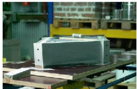
Figure 3.3 Demolding the diamond-shaped element made of textile-reinforced concrete.
