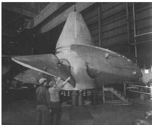
FIGURE 9.11 (a) Axial-flow propeller turbine. (b) Kaplan runner of an axial-flow turbine. (Courtesy of Allis-Chalmers Hydro Turbine Division. With permission.) (c) Typical installation of an axial-flow turbine system. (Courtesy of Allis-Chalmers Hydro Turbine Division. With permission.)
