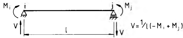
Fig. 4.24 Beam end moments and shears.
