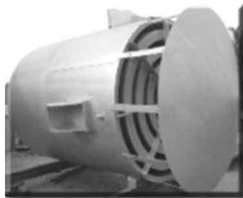
FIGURE 14.6 Safety valve vent silencer in manufacturer's shop.
