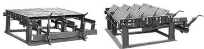
FIGURE 7.13 Small manual dumping grate assembly in shop floor in closed and dumping positions.
