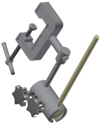
Figure 11.24. System for clamping the dummy, designed by the author and his team. For a color version of this figure, see www.iste.co.uk/grous/design.zip
