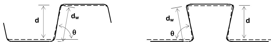
Figure 11.2b - Idealized section for sheet profile
