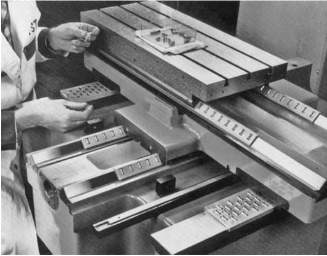
Figure 8-21 Flat linear roller guide of noncirculating type—CNC jig grinder (type G-18CP, late 1980s, courtesy of Moore Co.).
