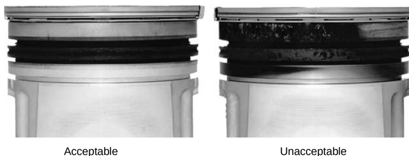
FIGURE 19.6 Detergents keep upper pistons clean.
