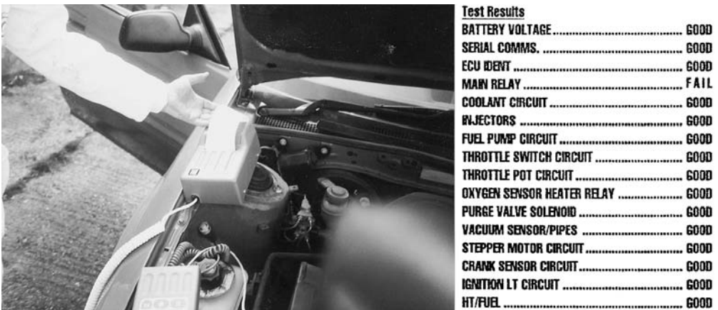
Fig. 3.18 The permanent copy of the test results
