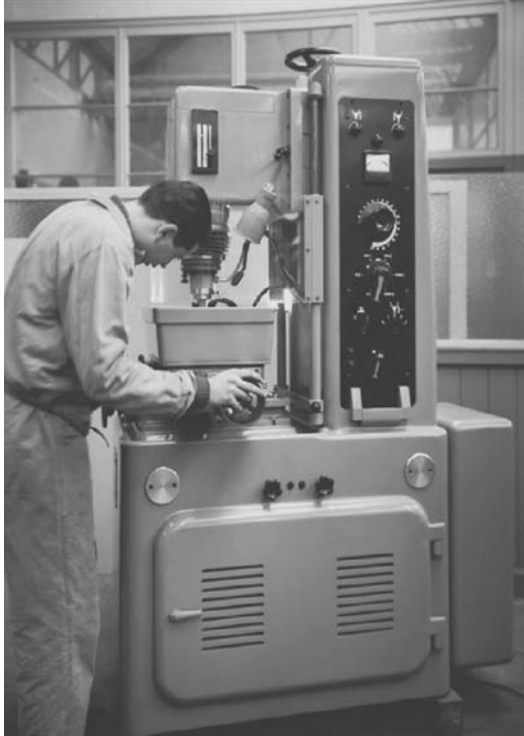
FIGURE 1.6 First industrial EDM machine in the world. Presentation of the Eleroda D1 at the EMO exhibition in Milan Italy, 1955. (Courtesy of Charmilles, 560 Bond St., Lincolnshire, IL.)
