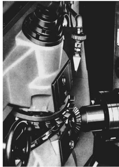
FIGURE 5.20 Bevel gear generating by interlocking cutters (Konvoid generators).
