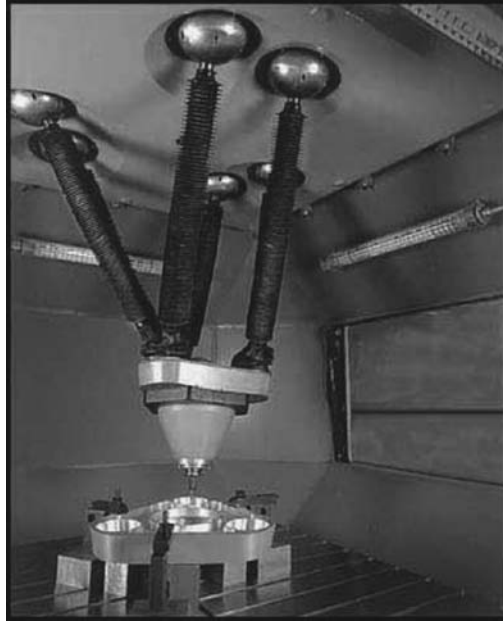
FIGURE 9.30 A typical hexapod machining application.
