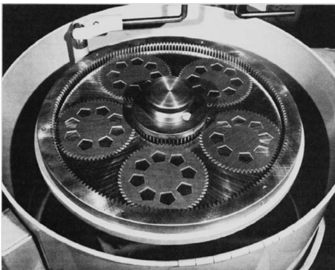
FIGURE 3.118 Planetary fixed-plate double-face lapping machine for flat surfaces. (From Hoffman Co., Carlisle, PA, USA.)
