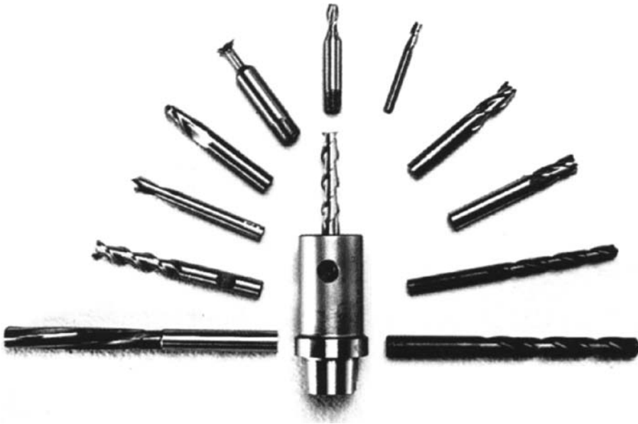
FIGURE 9.22 Tools accommodated by the spindle of a hexapod.
