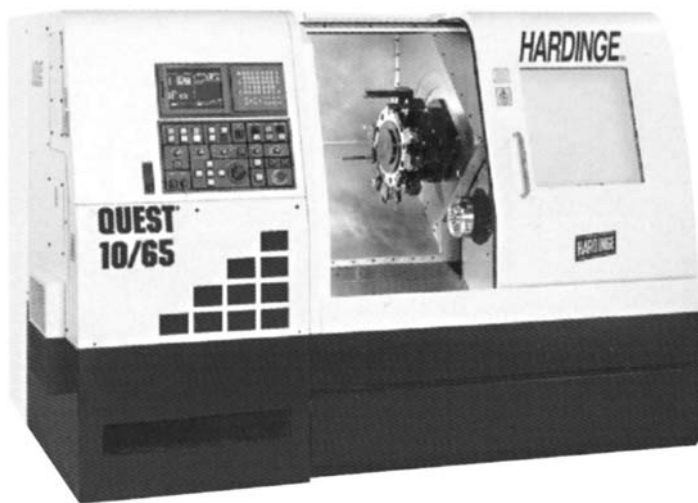
FIGURE 8.29 CNC lathe QUEST 10/56 of Harding Incorporation. (From Harding Inc. With permission.)
