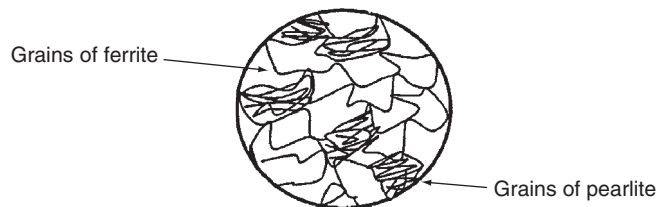
Figure 4.14 Microstructure of mild steel
