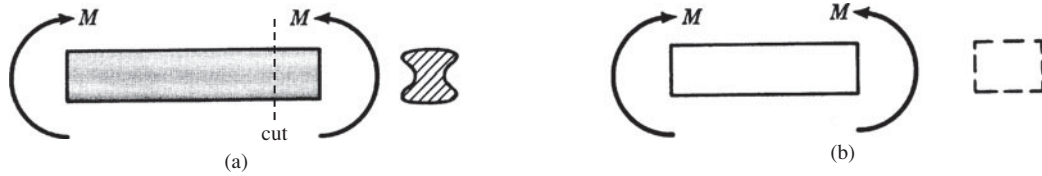
Fig. 7-2 A beam in pure bending.
