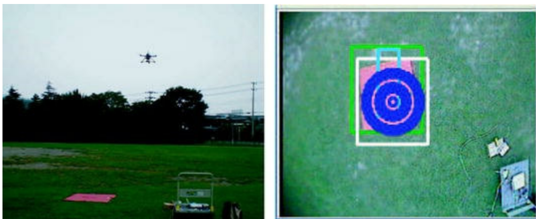
Fig. 10.11 Left: MAV hovering above target; Right: real-time tracking image by the onboard camera
