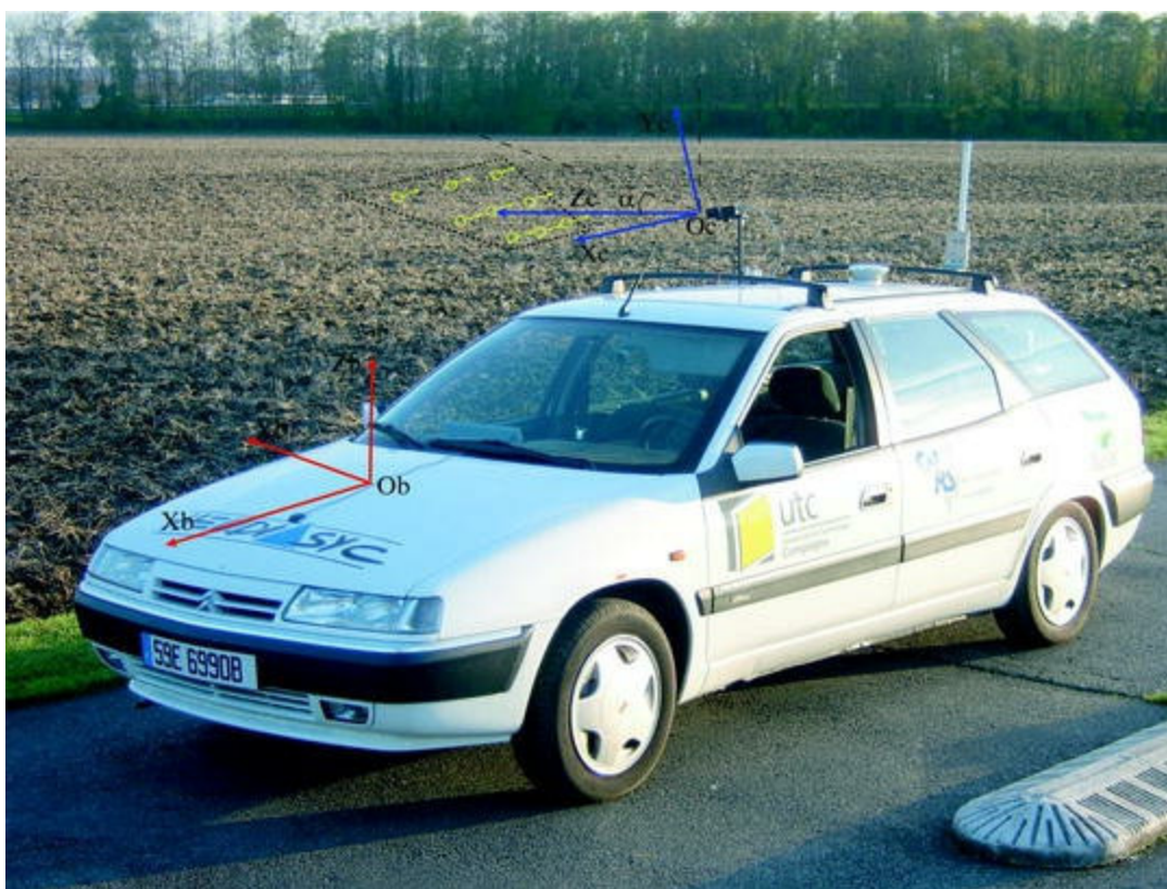
Fig. 10.3 The Heudiasyc intelligent vehicle (STRADA) in a forest road. The camera is mounted on the vehicle's roof and is looking laterally
