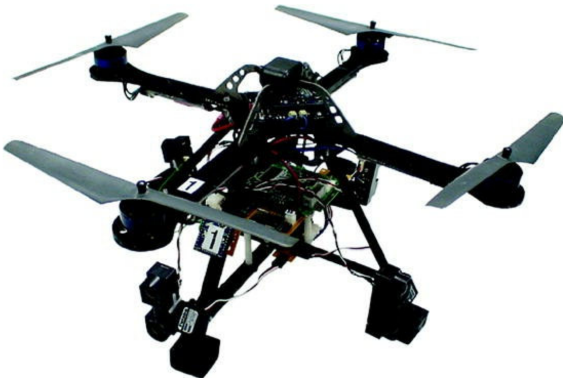
Fig. 13.1 Our autonomous quad-rotor flying robot for precise landing
