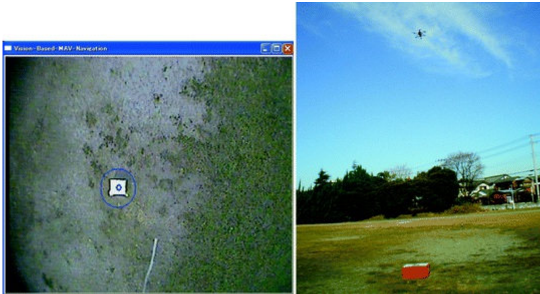
Fig. 12.9 Rotorcraft during vision-based autonomous hovering above a stationary target
