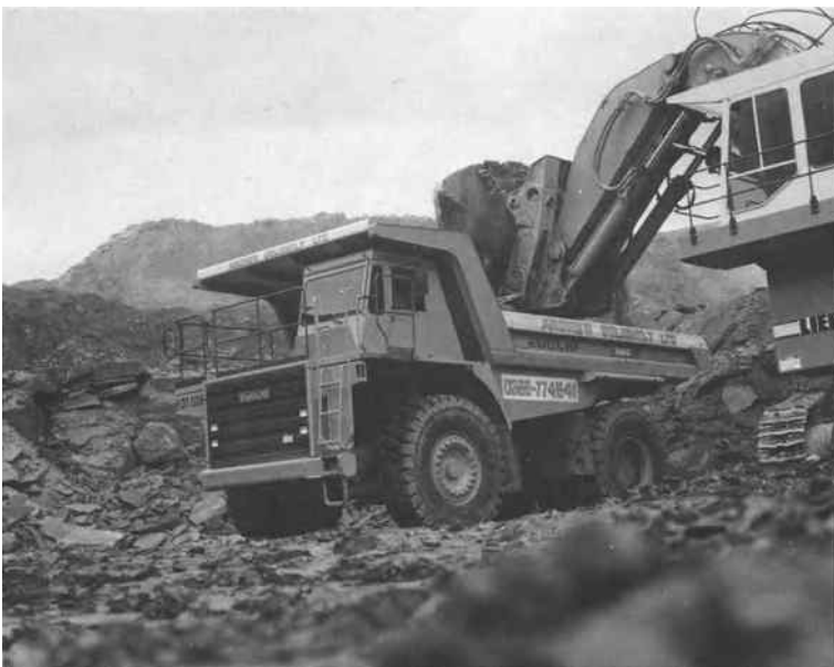
Plate 4b. A Euclid R60 522 kW dump truck, 36 m 3 heaped capacity. VME Construction Equipment GB Ltd, Duxford, Cambridge, UK
