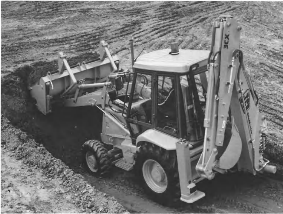
Plate 9a. The ubiquitous backhoe loader used on many sites. That shown is the JCB 3CX 56.5 kW, with shovel up to 2.3 m wide and hoe bucket 0.3–0.9 m wide. JCB Ltd, Rocester, UK
