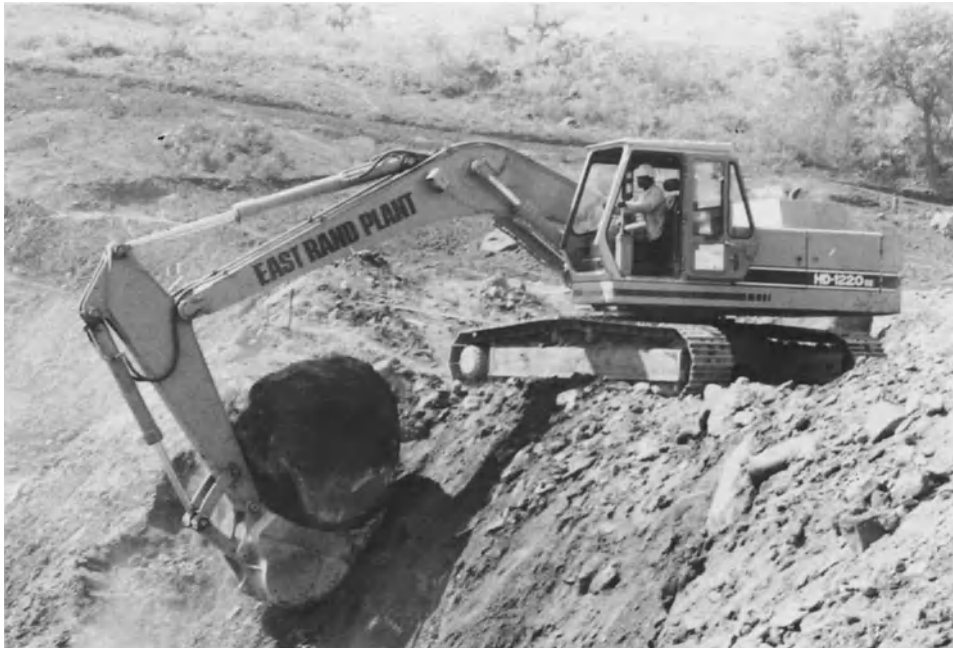
Plate 3b. A Kato 160 kW tracked excavator, with 1.6 m 3 bucket. ACP Holdings, Leicester, UK
