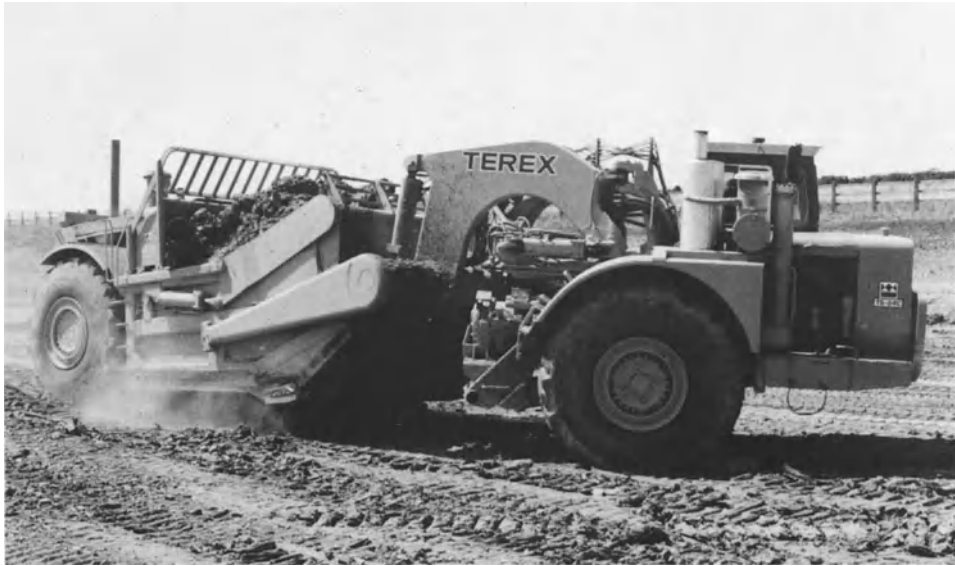
Plate 3a. A Terex TS24C 552 kW twin-engined 36 m 3 capacity scraper for earth-moving. Terex Equipment Ltd, Motherwell, Scotland
