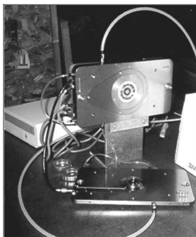
Figure 2 Modified shear apparatus for in situ SAXS/WAXD experiments. (Reprinted with permission from Somani RH, Hsiao BS, Nogales A, Srinivas S, Tsou AH, Sics I, Balta-Calleja FJ, Ezquerra TA. Macromolecules 2000;33(25):9385–9394. Copyright 2000, American Chemical Society.)
