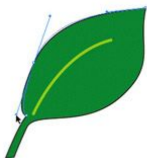
Figure 20-1: The depth and direction of Bézier curves are controlled by direction lines.
