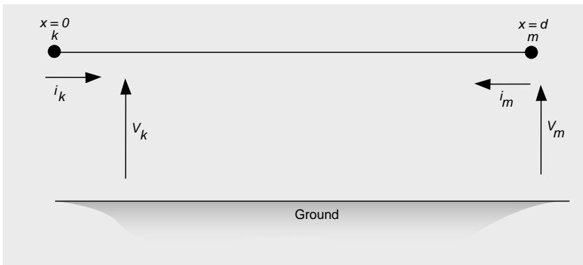
Figure 10.39 Transmission line with earth return
