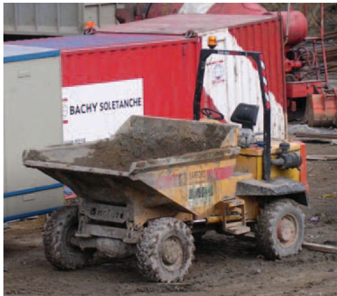
Figure 4.17 Dump truck with ROPS (arch over driving seat) fitted.
