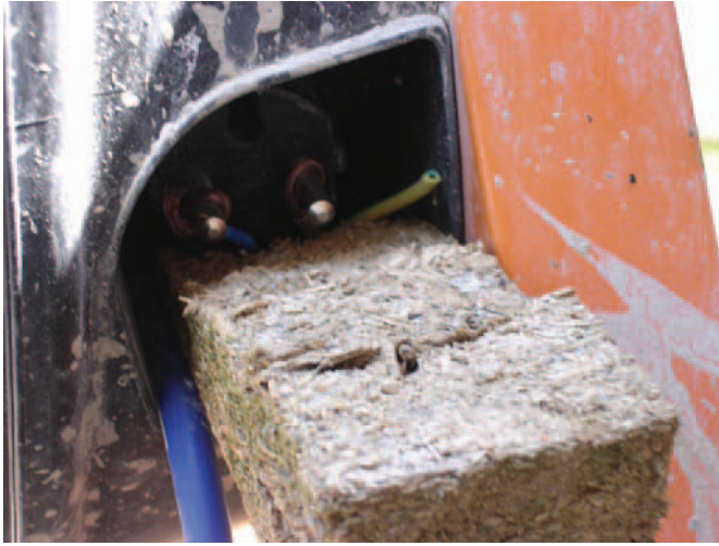
Figure 1.2 Dangerous electrics on cement mixer – the proper plug had been lost.
