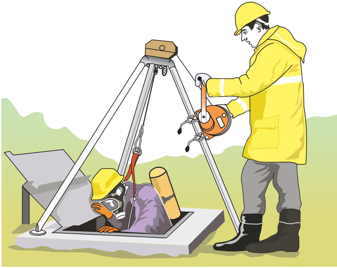
Figure 7.5a Confined space – method statement needed.
