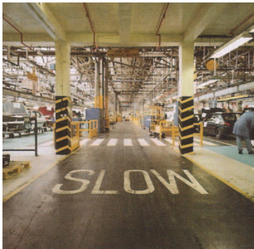
Figure 4.2 Well marked passageway in large factory with crossing point.
