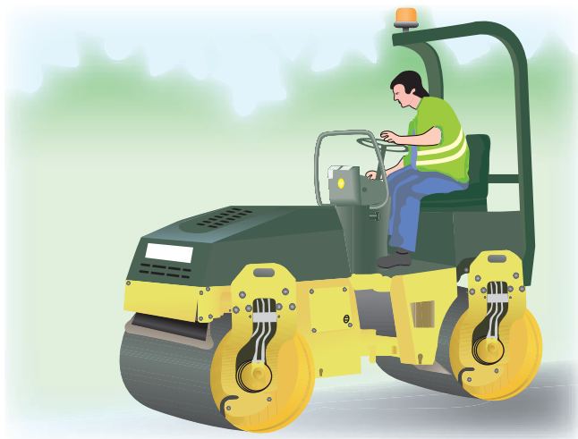
Figure 6.9 Vibrating roller potential for whole body vibration.
