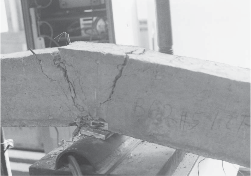
A plastic hinge in the maximum negative moment region.
