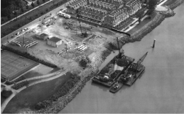
25.4 Ground densification using vibro-replacement at a river bank in Vancouver, British Columbia, Canada, to reduce the risk of liquefaction-induced lateral ground displacements (Wijewickreme et al. , 2005).
