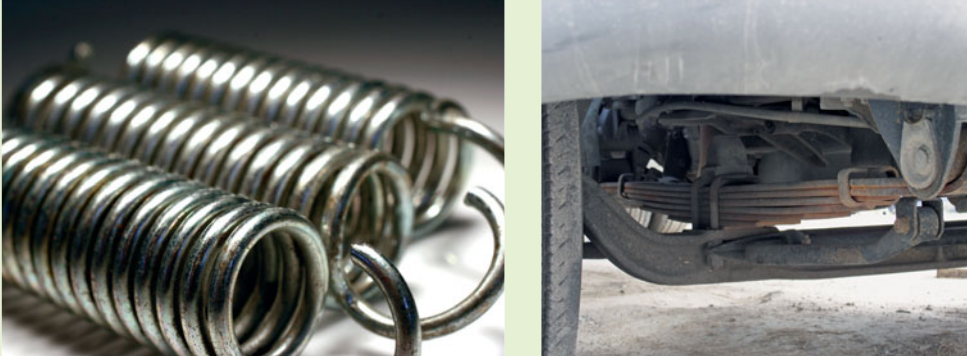
Figure 2.17 Images showing (left) helical or coil springs and (right) a leaf spring
