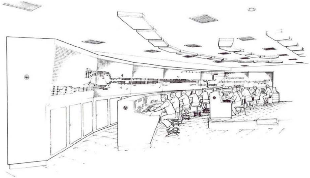
Fig. 5:3 Signalling control panel with separate operating console
