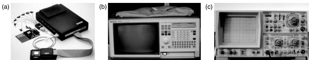
FIGURE 35.6 Tools for dynamic timing analysis. (a) Emulator, (b) logic analyzer, and (c) oscilloscope.
