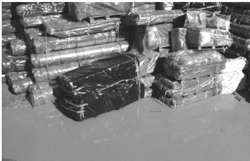
7.8 Cement-asbestos slates in a controlled landfill. During the disposal operations ACMs are often piled up in a messy way without care for package breakage or water contact necessary to prevent release of fibres in the air or water.
