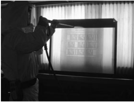
15.13 Technician cleaning plastic sheets with ink containing SWCNTs (courtesy Mary Schubauer-Berigan and Matt Dahm, NIOSH).
