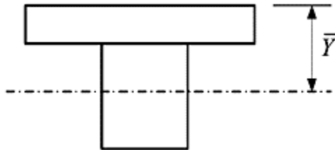
Figure 6.7 Depth of neutral axis for uncracked section for Example 6.2.
