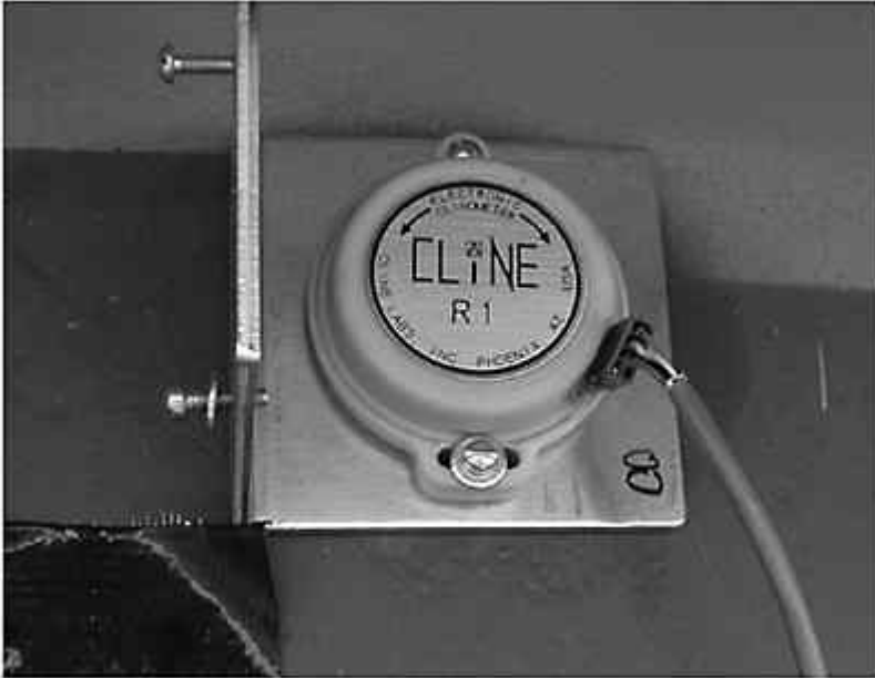
Figure 9.19 Inclinometer used to measure slope (Source: Copyright © (2008a) California Department of Transportation).
