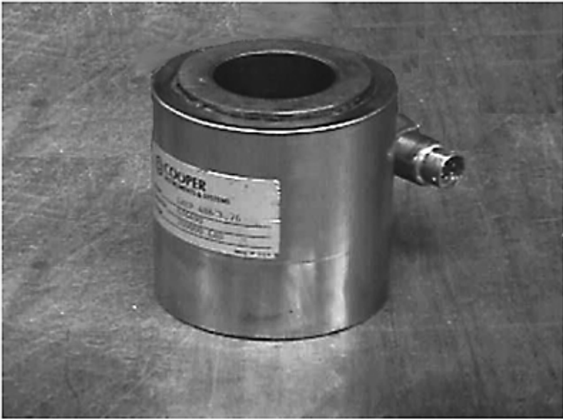
Figure 9.23 Load cells used to measure applied load.
