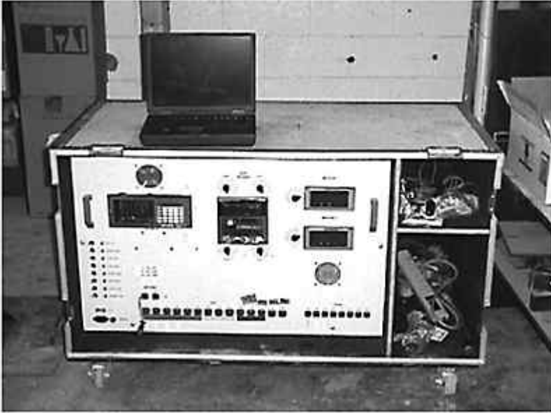
Figure 9.24 Data acquisition system collects data continuously from several devices.
