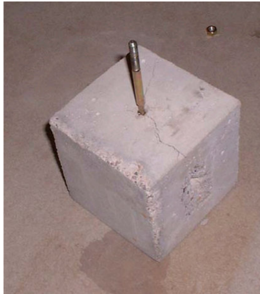
FIGURE 27.9 Test Cube After Pull-Out Test
