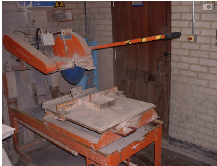
FIGURE 22.15 Chop Saw for Preparing the Ends of Cylinder Samples for Compression Test
