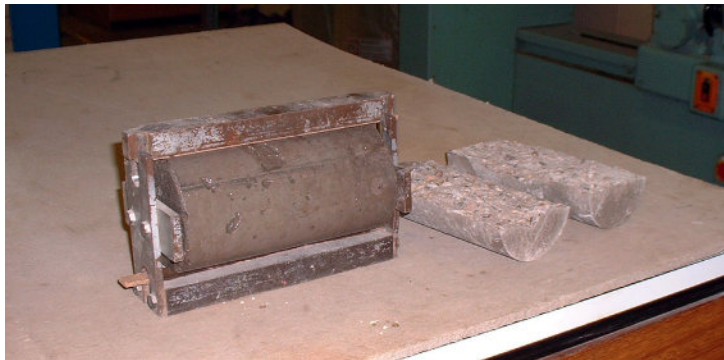
FIGURE 22.17 Cylinder Sample in Frame for Splitting, and Split Sample After Testing
