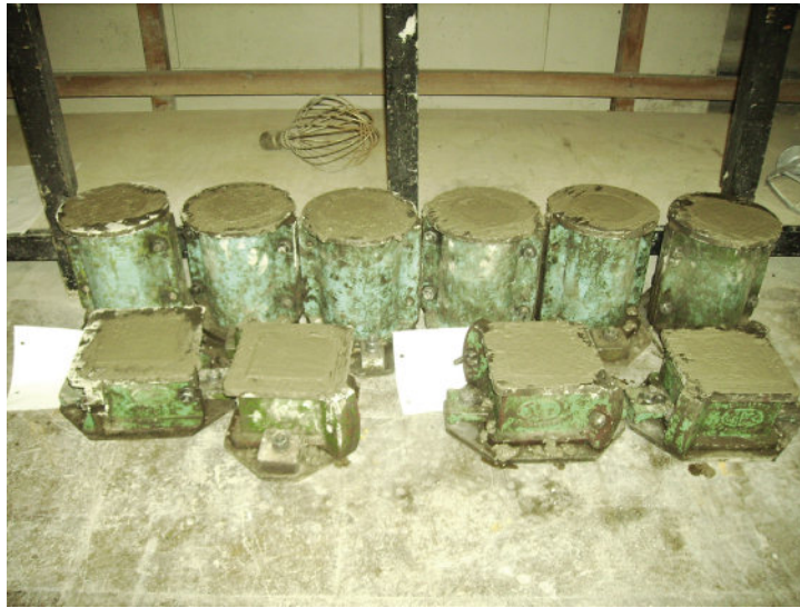
FIGURE 22.12 Filled Cube and Cylinder Moulds
