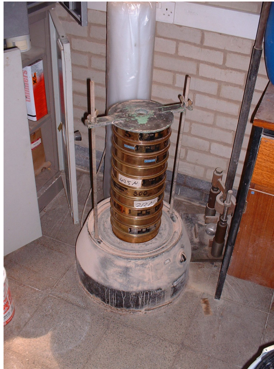
FIGURE 19.2 Sieves Stacked in Sieve Shaker
