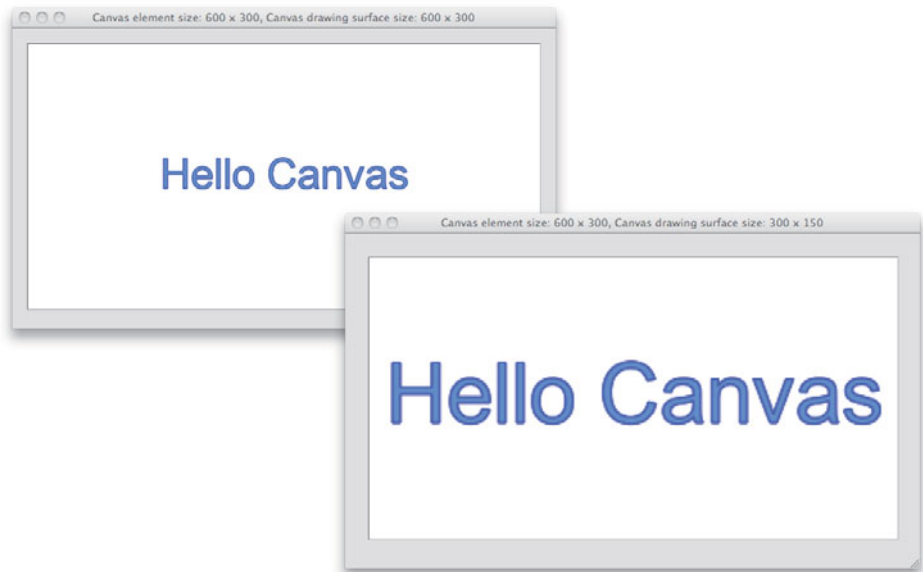
Figure 1.3 Top : element and coordinate system = 600 \times 300; bottom : element = 600 \times 300, coordinate system = 300 \times 150
