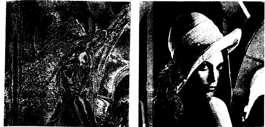
Fig. 13.19 A pseudo-greyscale image of a colour image 'Lena' (see Plate XIV) quantized to 256 colours. Left: palette ordered randomly (as created by the palette generation algorithm). Right: palette ordered along the luminance component of their colours.
