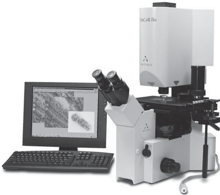
Fig. 1. Arcturus PixCell II Laser Capture Microdissection System. The Arcturus system uses an infrared laser to melt a polymer into the tissue sample. When the laser pulse is completed, the polymer solidifies and will lift out the captured cylinder of tissue.
