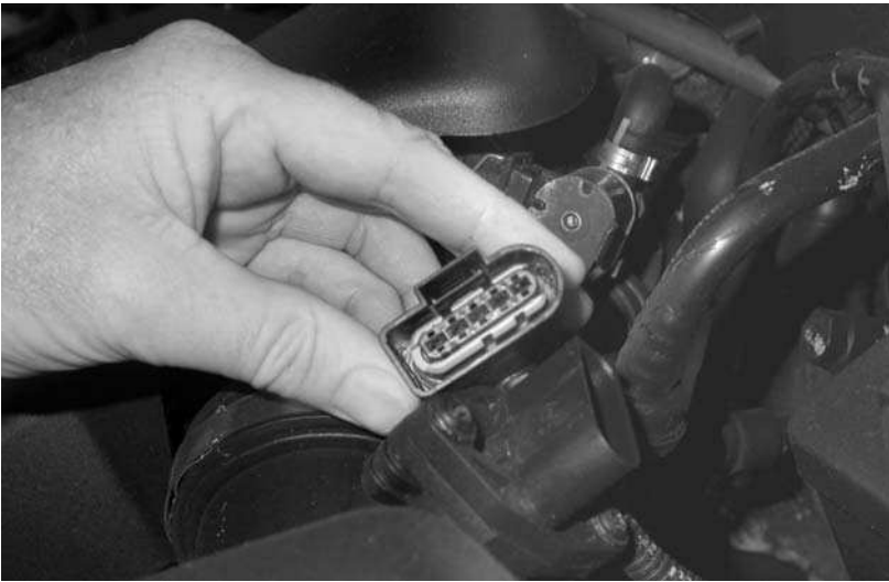
Figure 7.43 Air flow meter under test
