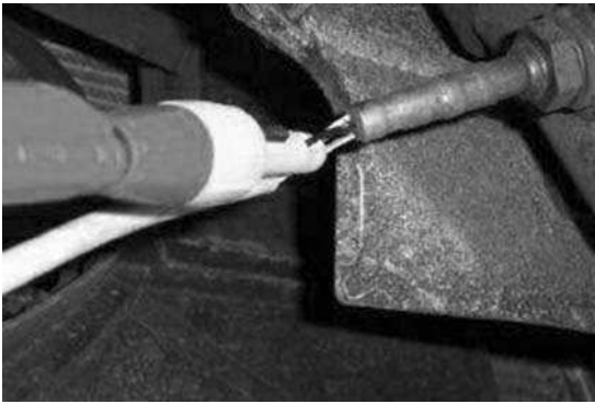
Figure 4.16 Titania knock sensor in position
