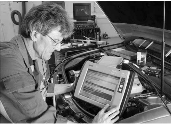
Figure 3.15 Diagnostic system in use (Source: Bosch Press)
