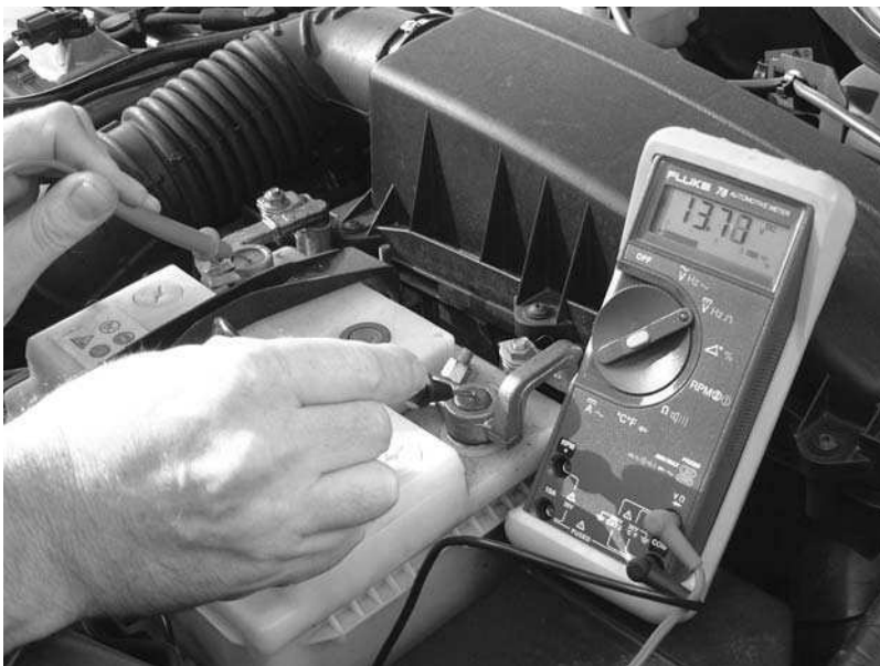
Figure 7.57 Battery voltage testing
