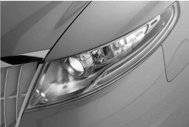
Figure 9.11 Adaptive lighting using LEDs
