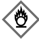
Flame Over Circle (oxidizing hazards)
