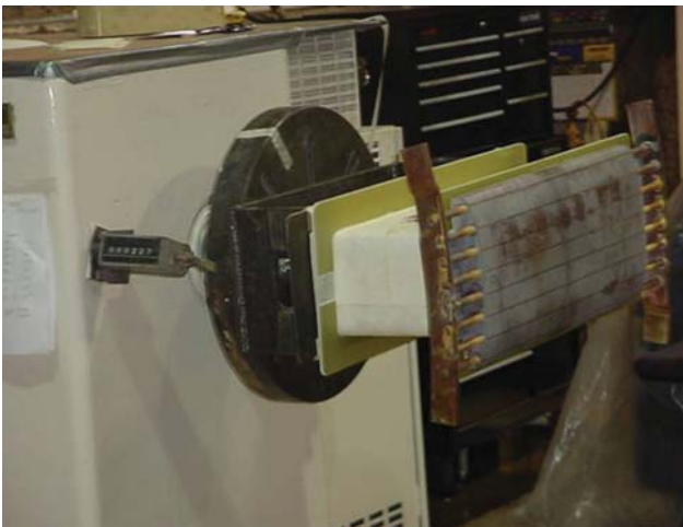
Figure 18.12 Resin-impregnated wire-wound pole windings.
