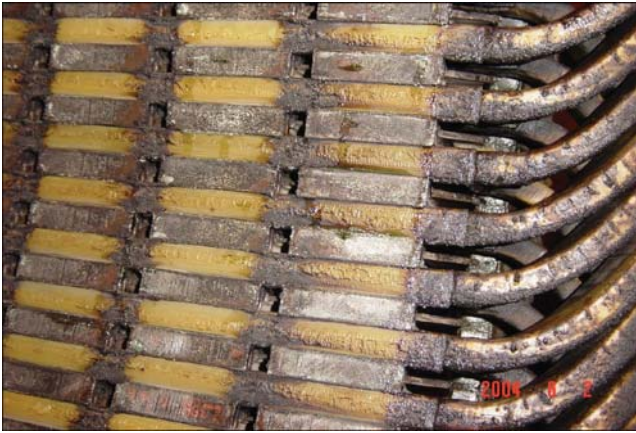
Figure 8.18 Photo of a stator winding degraded by acids in chimney flue gas.
