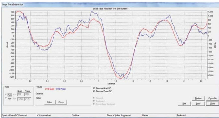
Figure 17.20 El-CID QUAD and PHASE current comparisons along a stator slot at a core split—same shape and constant PHASE/QUAD current ratio confirms that there is no core insulation damage. (Source: Courtesy Iris Power-Qualitrol.)
