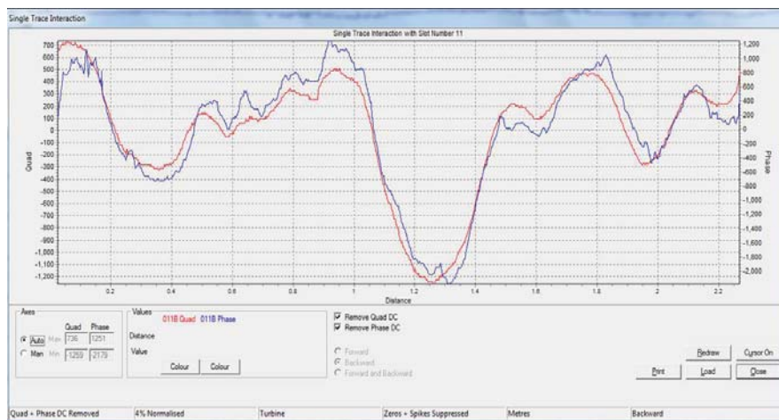
Figure 17.20 El-CID QUAD and PHASE current comparisons along a stator slot at a core split—same shape and constant PHASE/QUAD current ratio confirms that there is no core insulation damage. (Source: Courtesy Iris Power-Qualitrol.) See color plate section.
