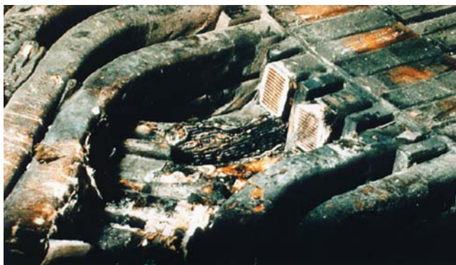
Figure 8.14 A turn-to-turn failure leading to a ground fault on a 6.6 kV, 8 MW motor. A bottom coil experienced the failure, and the top coils were cut away to expose the fault.
