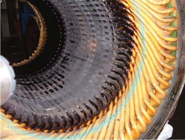
Figure 13.1 Blockage of stator core ventilation ducts with dirt and oil.
