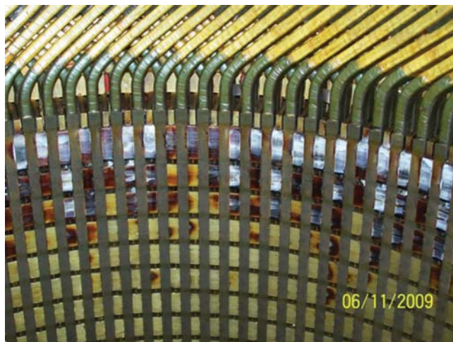
Figure 13.2 Stator core burning that resulted from excessive oven temperatures during stator winding burnout prior to rewind.
