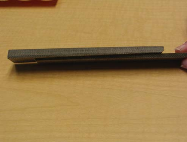
Figure 1.15 Side view of a two-part wedge, where a tapered slider is pushed under the wedge to increase radial pressure on the coils.
