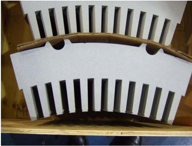
Figure 6.3 Segmented stator core laminations used in large diameter stator cores.
