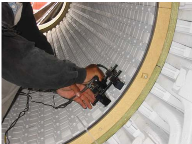
Figure 17.15 El-CID trolley with Chattock coil mounted.
