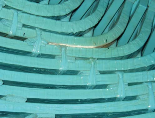
Figure 8.20 PD between adjacent coils in different phases results in white powder on the stator bar surfaces. (See color plate section).
