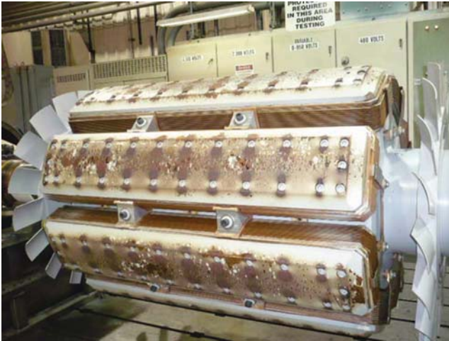
Figure 18.11 Laminated pole with ground insulation and pole washers installed ready for wire winding.
