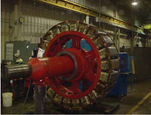
Figure 1.3 Photograph of a salient pole rotor for a large, low speed motor (Source: Photo courtesy Teco-Westinghouse).
