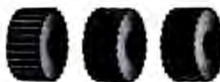
Knurls (left to right): A straight tooth knurl, left hand and right hand 30° spiral knurls.
