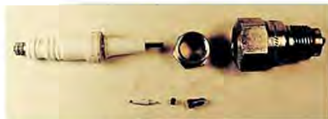
At the top is a real spark plug, below it is a 1/5 scale working model by Jerry Kieffer. Below is a closer look at another small spark plug and its components.
