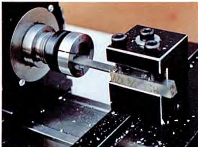
(Above) A pot chuck is being turned to the proper inside diameter to grip a particular diameter part.
