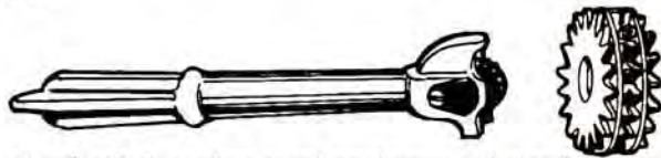
A wheel dressing tool and spare "star" cutter
