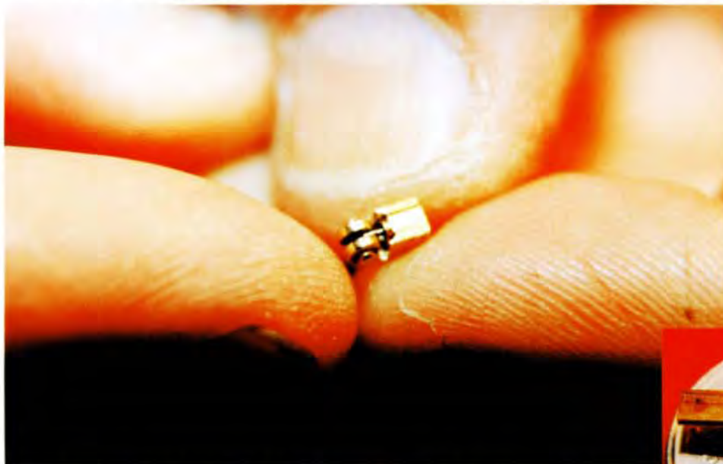
Even Jerry Kieffer admits that he is "pushing his limits" with this tiny oscillating steam engine. It has two flywheels .085" in diameter. The bore is .029" and the stroke is .032" The intake and exhaust ports are .008" and the whole engine weighs 3.5 grains ( 1/131 oz.)
