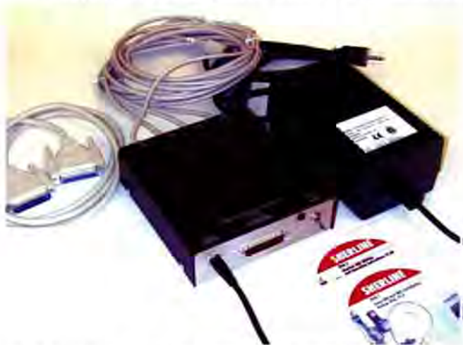
A driver box like this Sherline P/N 8760 4-axis box makes it possible to drive stepper motors from any PC computer. Cables plug into the X, Y, Z and A axis stepper motors. A 25-pin cable goes to the computer's parallel port. A power supply is included.
