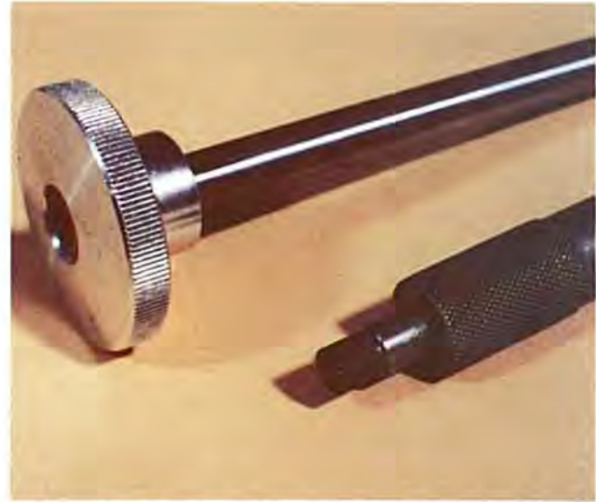
This collet drawbar has a straight knurl while the micrometer handle uses a diamond pattern. Each provide good grip and a professional looking appearance. The knurling process embosses the pattern into the metal rather than cutting it.
