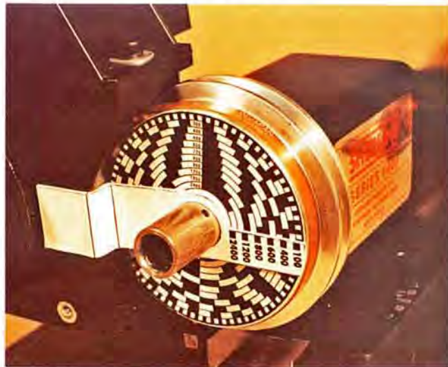
The RPM gage and indicator mounted to a lathe. Though sized for a Sherline pulley, the gage may be resized for use in other applications as well.
