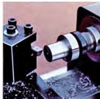
(Above) A pot chuck is being turned to the proper inside diameter to grip a particular diameter part.
