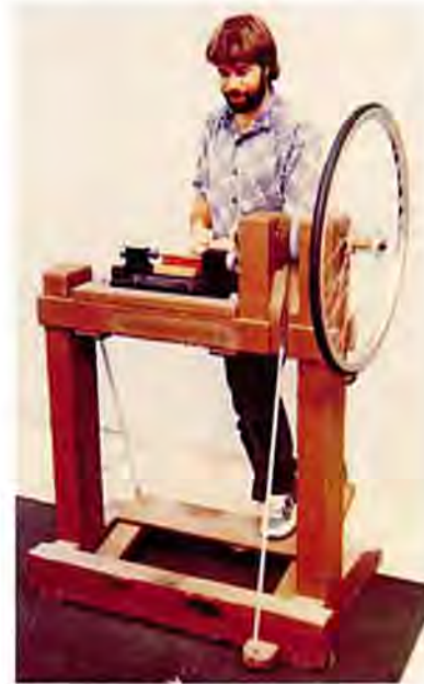
Chip Ivester and his "missing link" foot powered lathe for wood turning. Some samples of Chip's work can be seen on page 41.
