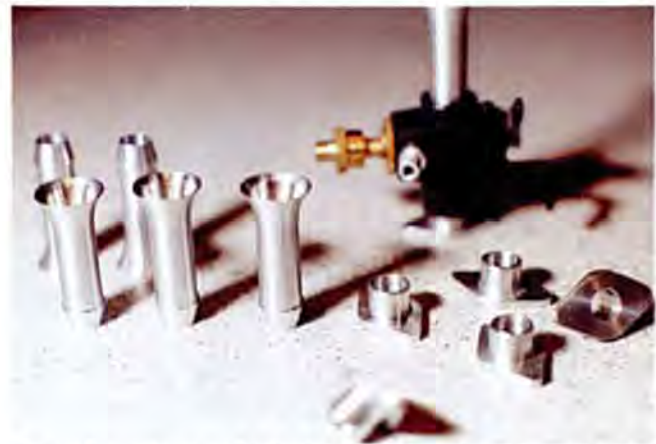
A carburetor and air inlet tubes for Pete Weiss' miniature Porsche engine project.
