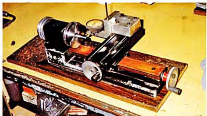
Sherline uses some of their own tools for small jobs in their production line. Shown here are a number of special tools used for making chucks and collets. Clockwise from top left: Drilling tommy bar holes, grinding inside of chuck jaws, checking chuck runout and a setup to center drill, drill, ream and face collets.
