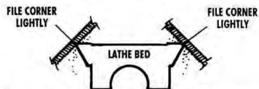
Filing corners of bed dovetail for better fit of Tailstock Riser Block.
