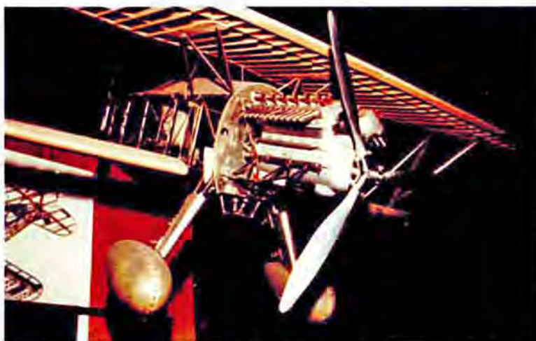
Alan Ingersoll’s 1:6 scale Curtiss P6-E biplane is shown uncovered so the construction detail can be appreciated. It will be displayed in the Hiller Aviation Museum in San Carlos, California. The project took over 12 years to complete.
