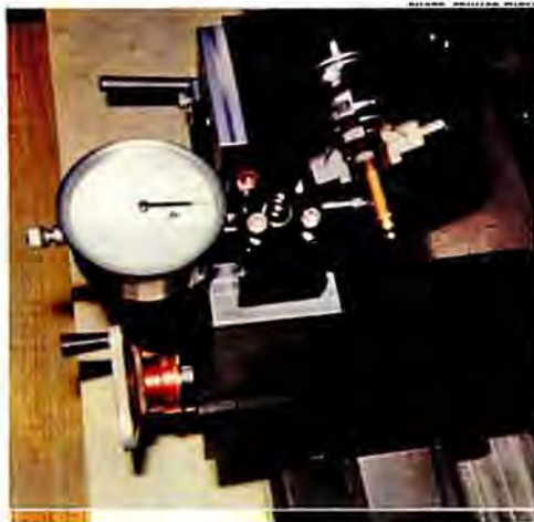
Mr. Ewell's setup with the dial indicator being held in the 3/8" hole of the P/N 7600 toolpost.
