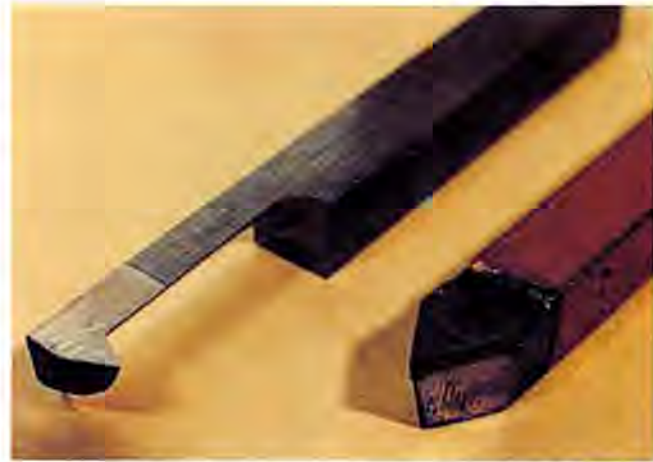
A 1/4" tool used for cutting inside threads (left) and a 60^\circ carbide thread-cutting tool (right).
