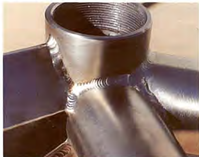
Some welding shops specialize in exotic metals. Welding titanium such as this Mako mountain bike frame requires special tools and a lot of skill. The advantage gained here is a frame that weighs 2.5 pounds instead of the 5 pounds it would weigh if made from steel.
