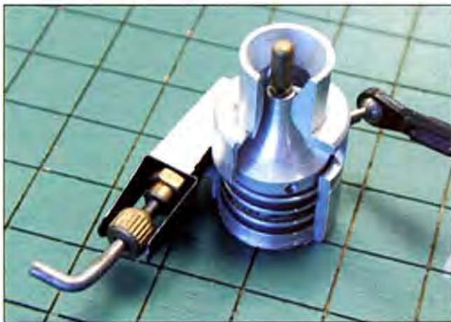
The M-H variable venturi carburetor for model aircraft engines earned a patent of limited value.
