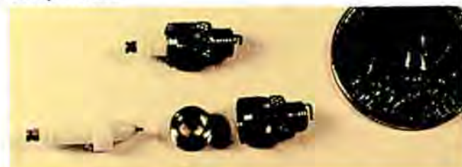
At the top is a real spark plug, below it is a 1/5 scale working model by Jerry Kieffer. Below is a closer look at another small spark plug and its components.
