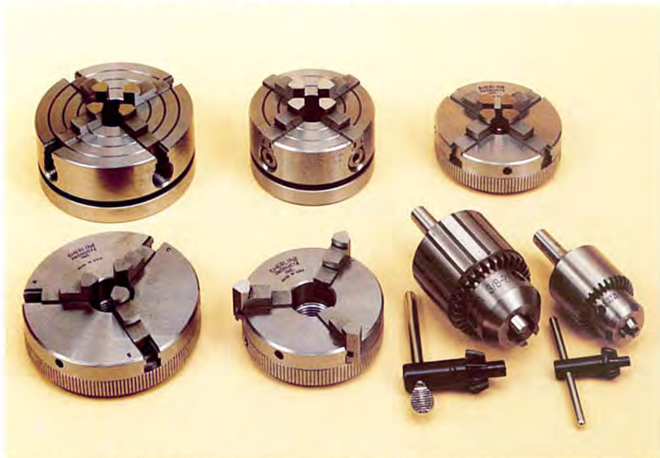
3-jaw, 4-jaw and tailstock chucks of various sizes for use on Sherline tools or any tool with a 3/4-16 spindle nose thread. Other threads are available to allow the chucks to be used on some Unimat, Sears and Cowells lathes. Arbors are also available to adapt them for use on watchmakers lathes. The 2.5" 3-jaw chuck in the middle of the bottom row is shown with its jaws reversed for holding larger work.
