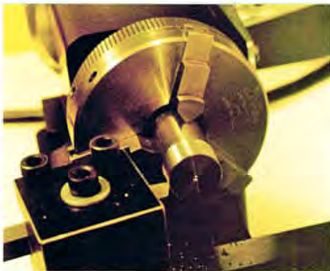
A part is shown held in a 3-jaw chuck. The 3-jaw chuck is easy to use and is the single most popular accessory for Sherline tools.
