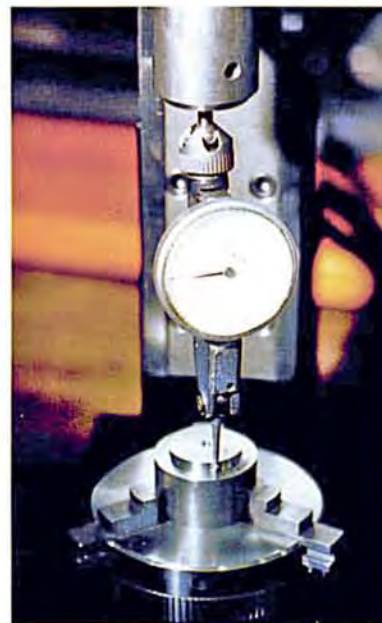
(Right) Indicating in the surface of the flywheel for milling. The part is left in the 3-jaw chuck so it can be returned to the lathe for parting off without recentering.
