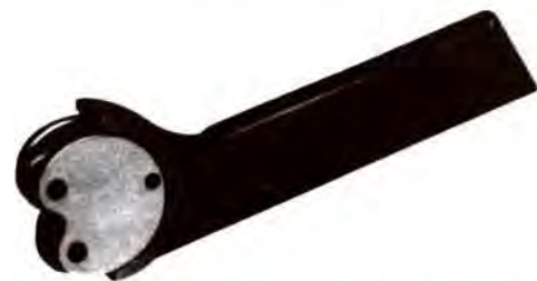
A knurling tool used for "bump knurling" in a standard size lathe. It is held in the toolholder and pressed into a firmly supported rotating part.
