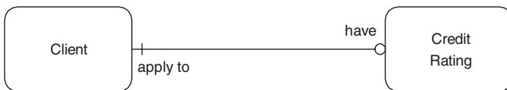
Figure 10.19 Separate entity class for credit rating attributes.
