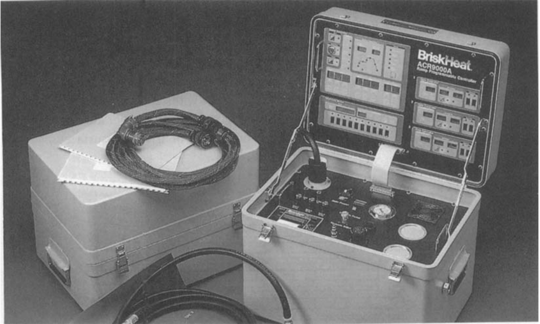
Fig. 10.3.5 Second Generation BriskHeat ACR9000 Ramp Programmable Controller, Circa 1990
