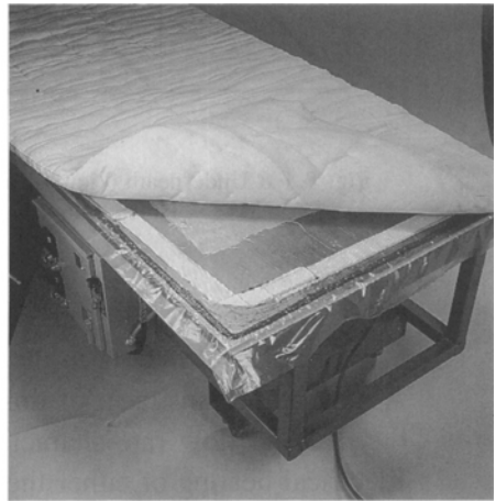
(c) Experimental complex curvature vacuum blanket up to 450°F
