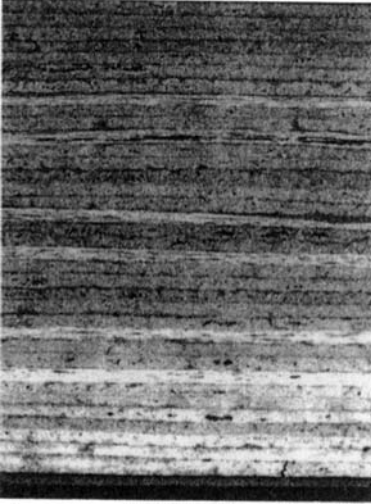
Fig. 9.3.2 Voids and Porosity
