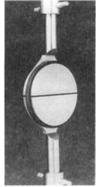
(c) Split disc tensile fixture is used for testing reinforced plastic rings.
