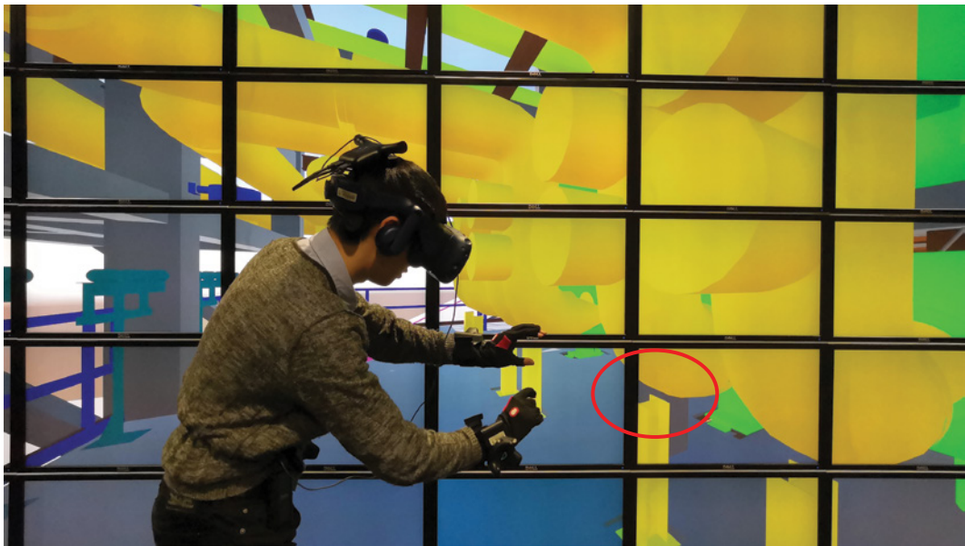
FIGURE 10.4 Design review session in virtual reality—missing support for a pipe spool
