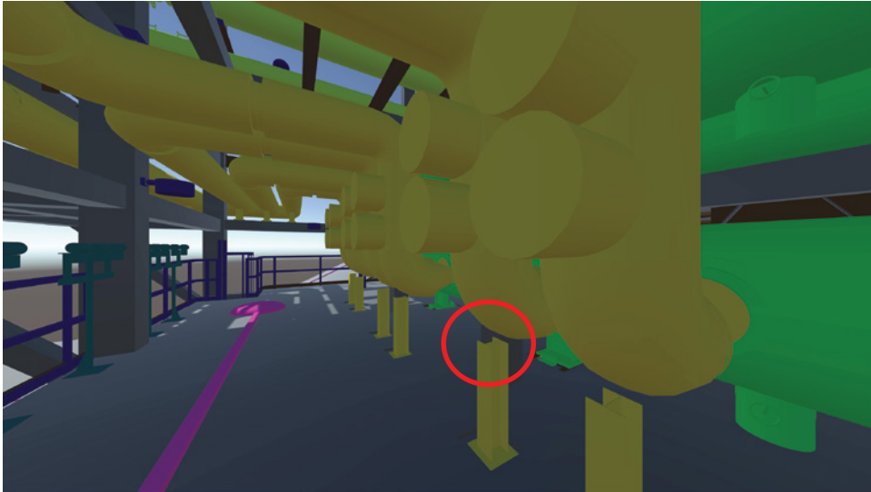
FIGURE 8.7 Missing support for pipe spool (false negative)
