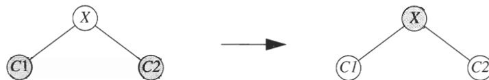
Figure 19.38 Color flip: Only if X 's parent is red do we continue with a rotation.
