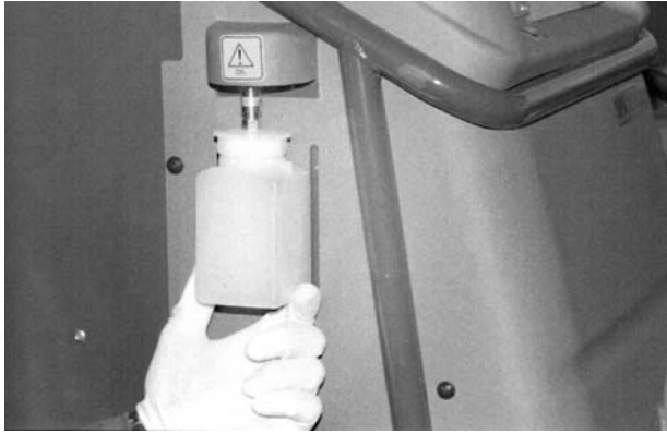
Figure 5.21 Oil being added while the system is under vacuum
