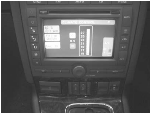
Figure 3.91 Touch screen display (TFT LCD) which communicates with A/C module (module not built in)
