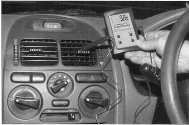
Figure 5.15 Centre vent temperature check
