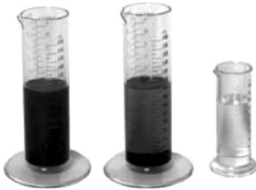
Figure 5.31 Examples of flushed material (courtesy of Autoclimate)
