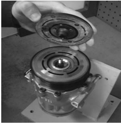
Figure 5.34 Slide armature up and off shaft
