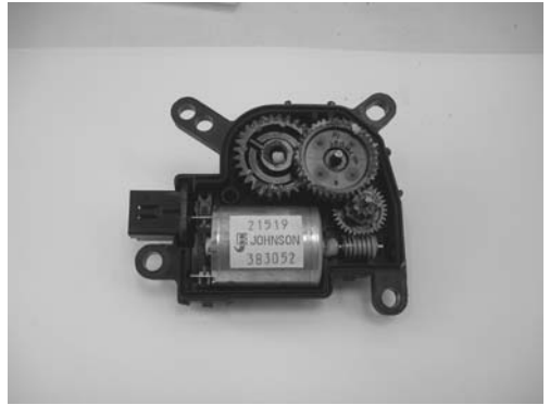
Figure 1.29 Electrical control motor and reduction gear
