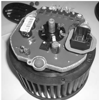
Figure 3.73 Voltage applied to stator coil by control circuitry
