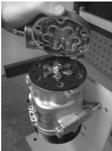
Figure 5.52 Removal of cylinder head
