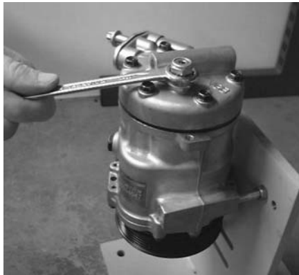
Figure 5.57 Removal of high pressure relief valve
