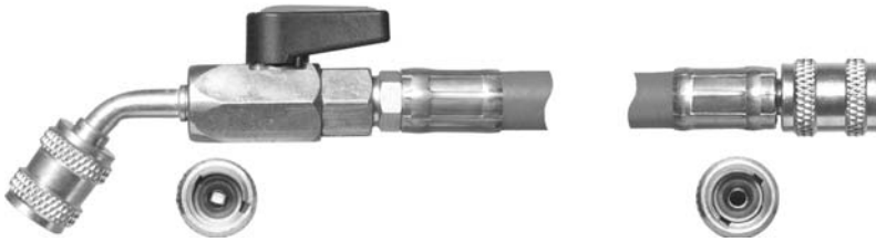
Figure 1.47 R12 low pressure connector 1/4" SAE Schrader valve 45° end fitting with Goodyear GY5 barrier hose (courtesy of Autoclimate)
