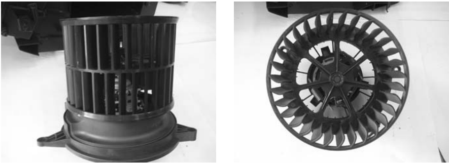
Figure 1.16 Centrifugal type fan assembly
