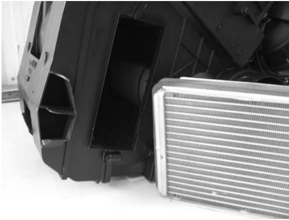
Figure 2.42 Location of an evaporator inside the heater box
