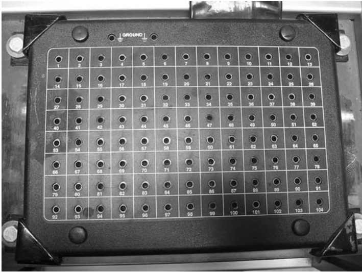
Figure 3.103 104 pin break-out box (without serial interface)
