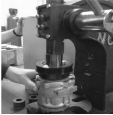
Figure 5.41 Installation of rotor using arbor press
