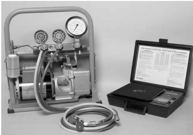
Figure 5.2 A portable charging unit with vacuum pump and scales. This unit can vapour charge or liquid charge using a heat belt or charging cylinder
