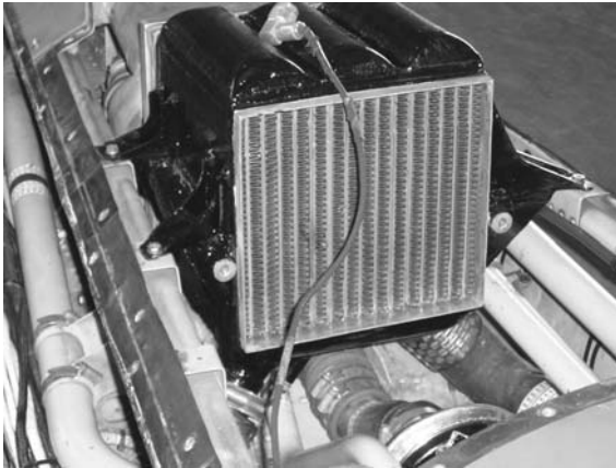
Figure 1.63 Secondary heat exchanger (courtesy of RAF Coltishall)
