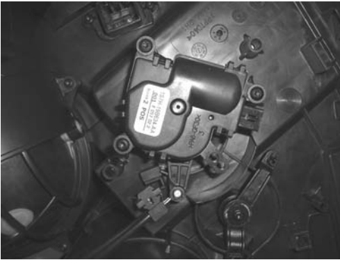
Figure 1.29 Electrical control motor and reduction gear
