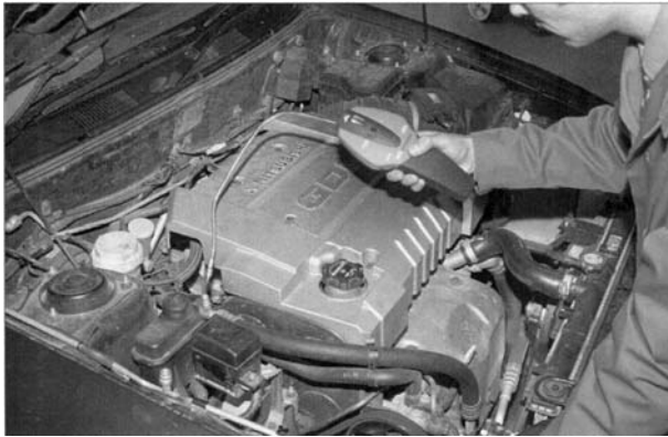
Figure 5.23 Check all refrigerant pipes, hoses and seals for leaks
