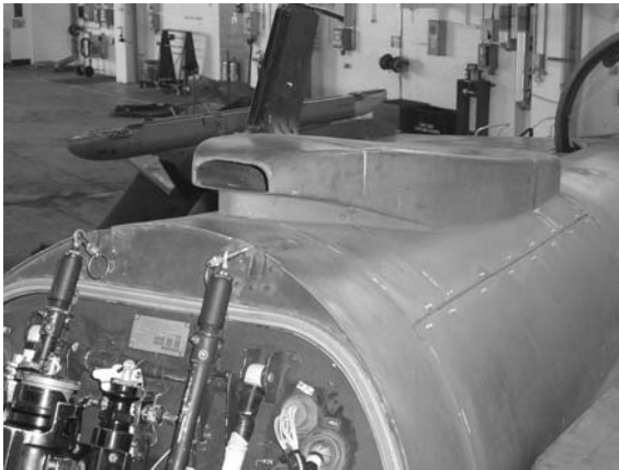
Figure 1.62 Secondary heat exchanger inlet (courtesy of RAF Coltishall)
