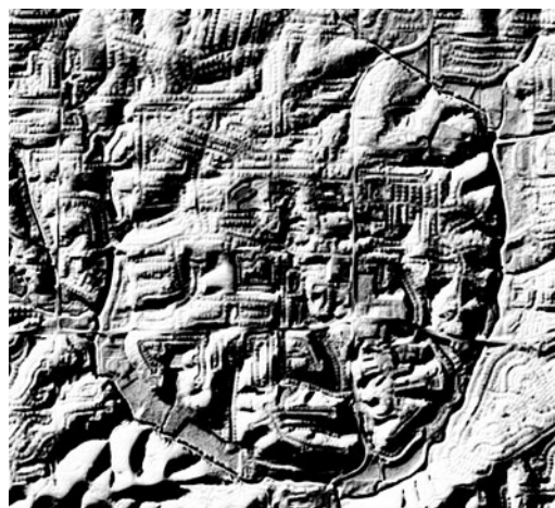
LiDAR digital elevation data shown here with hillshading reveals topographic information used for hydrologic modeling (Photo courtesy Vieux and Associates)
