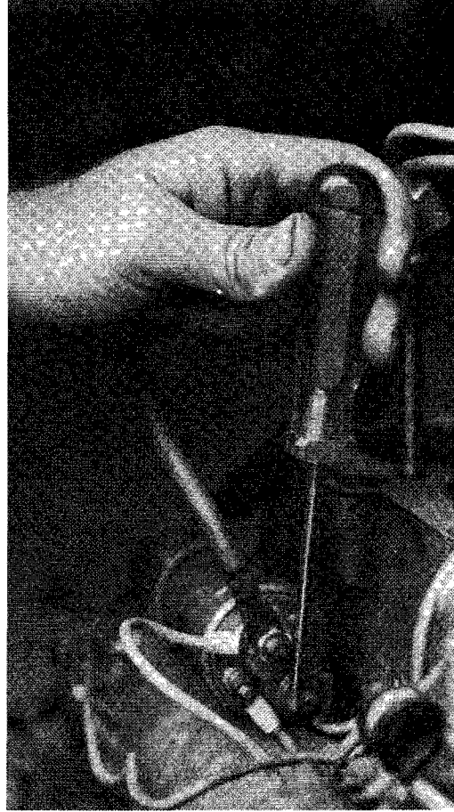
By-passing the solenoid altogether by jumping out the two main cable terminals.
