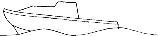
The same boat moving at 7½ knots. There will be approximately one wave to its length. This boat is moving at hull speed for displacement boats of that length.
