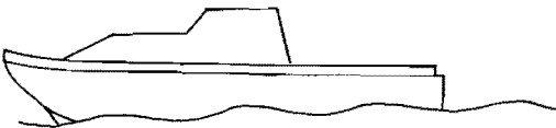
A 32-foot (waterline length) boat moving at 4 knots. There will be approximately 3½ waves to its length.
