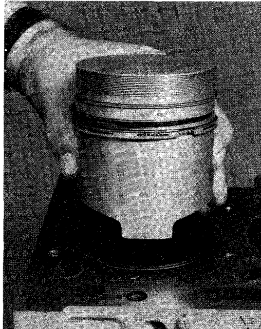
Figure 11-56. Lowering a piston into its cylinder. (Courtesy Perkins Engines Ltd.)
